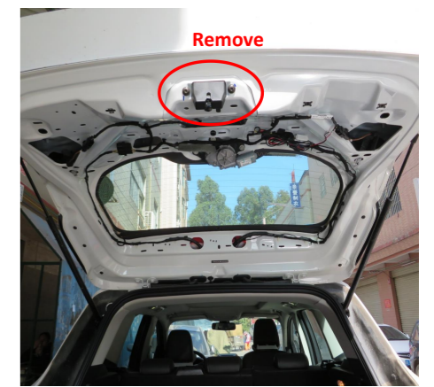
6. Remove the original latch.
