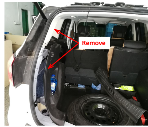
4. Take out the trunk floor mat and remove the trim panels on the left side of the trunk.
