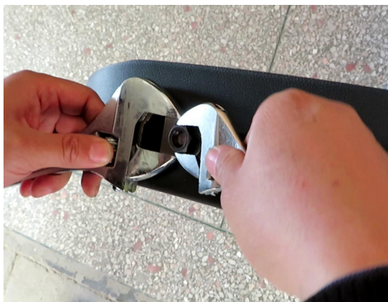
27. Open the hole (one hand secures the hole opener and the other hand turns the wrench).
