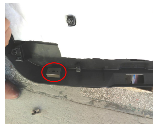
24 Place the base of the hole opener at the indicated position of the tailgate trim panel.
