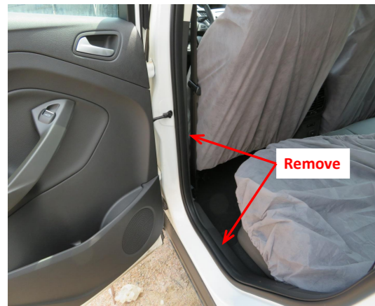
2. Remove the rear left side door sill panel and B-pillar trim panels.
