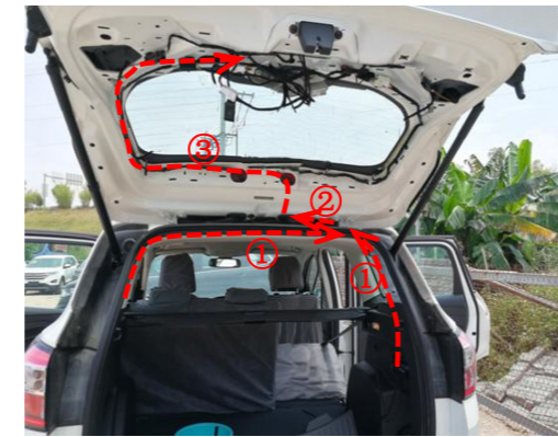
14. Route the power harness to the tailgate (do not connect plugs before inserting terminals into wiring harness connector).
