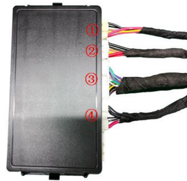
22. Insert the strut wiring harnesses ①②, lock signal harness ③, and power harness ④ into the ECU in sequence and the ECU onto its bracket.
