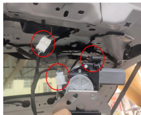
8. Connect the lock signal harness to the plugs of the power latch and the added tailgate switch.
