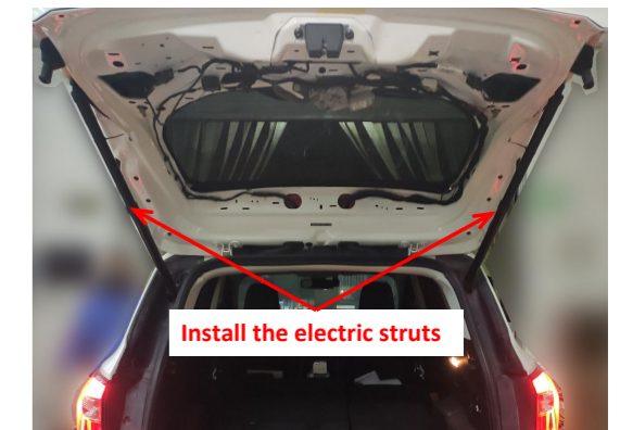
11. Install the electric struts, L on the left and R on the right (the first letter of the strut code), making sure the ends with wiring harnesses are on the tailgate.
