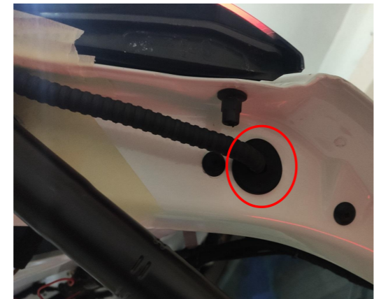
13. Plug the holes with hole plugs.
