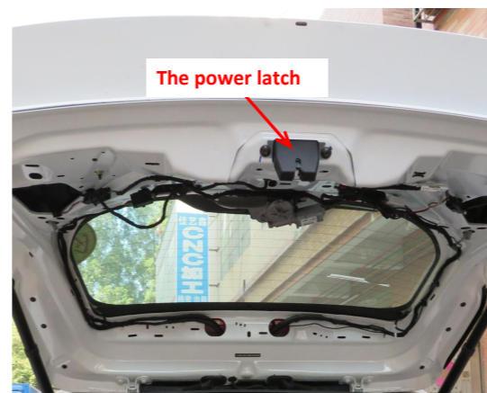
9. Install the our power latch.
