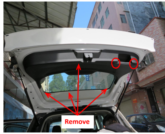
3. Remove the tailgate trim panels.
