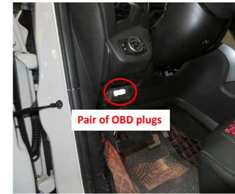
20. Connect the power harness to the OBD plug (remove the OBD plug from the slot and hide the pair of plugs inside).
