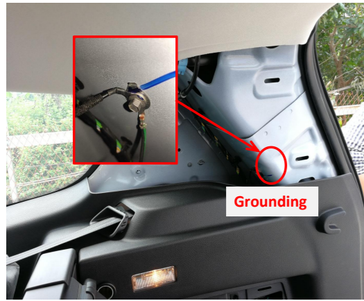
17. Ground at the right side of the trunk.
