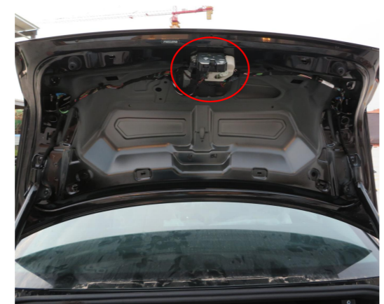
13. Remove the original latch.
