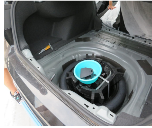
4. Remove the trunk floor mat and the door sill trim.
