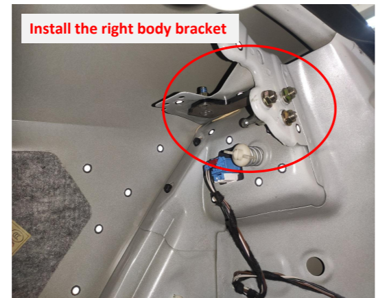
8. Install the right body bracket.
