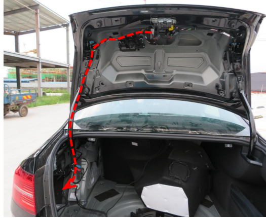
17. Route the lock signal harness to the left side of the trunk through the left hinge.
