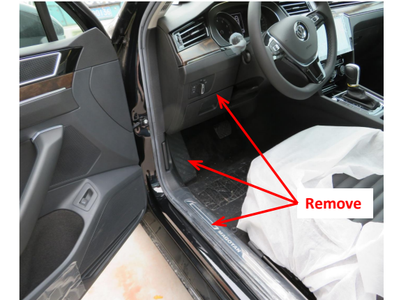
1. Remove the front left door sill trim, switch panel and the rest pedal.
