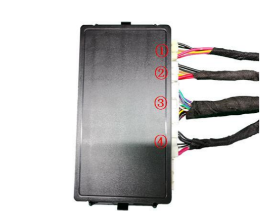
25. Insert the strut wiring harnesses ①②, lock signal harness ③, and power harness ④ into the ECU in sequence.
