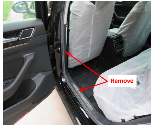
2. Remove the rear left door sill trim and B-Pillar trim.
