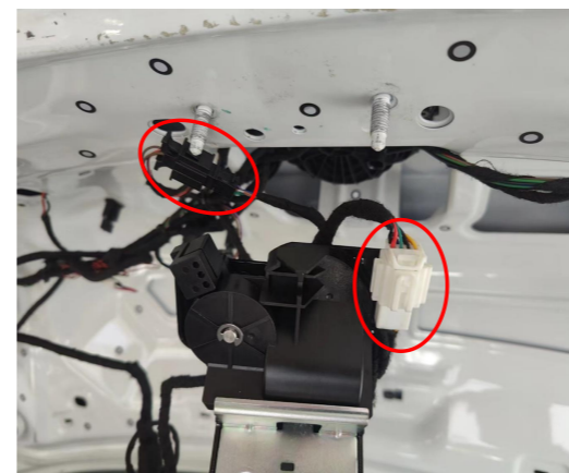
14. Connect the plugs of the lock signal harness to the power latch .
