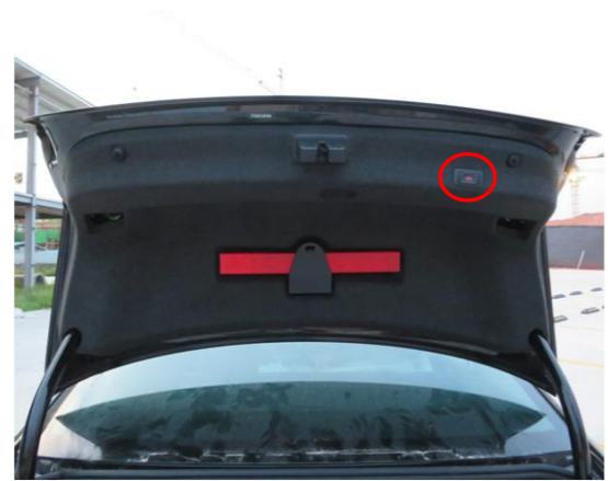
28. Install all the trim panels back and install the added tailgate switch.
