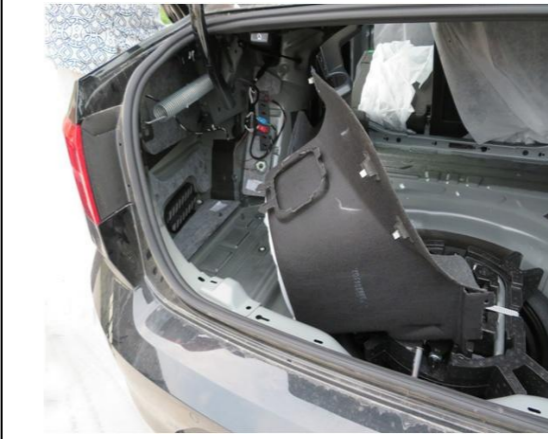
5. Remove the trunk trim on the left and right sides and fold the rear seat.
