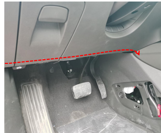
22. Route the pink plug to the left side of the passenger seat.
