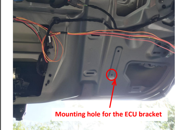
26. Install the ECU bracket at the indicated hole.
