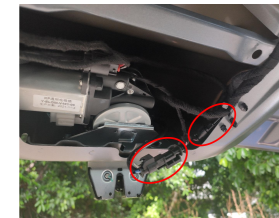
10. Connect the lock signal harness to the plugs of the original handle switch.
