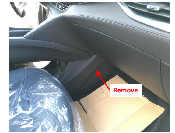
1. Remove the indicated trim panel on the left side of the front passenger position.
