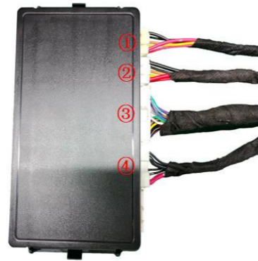
28. Insert the strut wiring harnesses ①②, lock signal harness ③, and power harness ④ into the ECU in sequence and mount the ECU onto its bracket.
