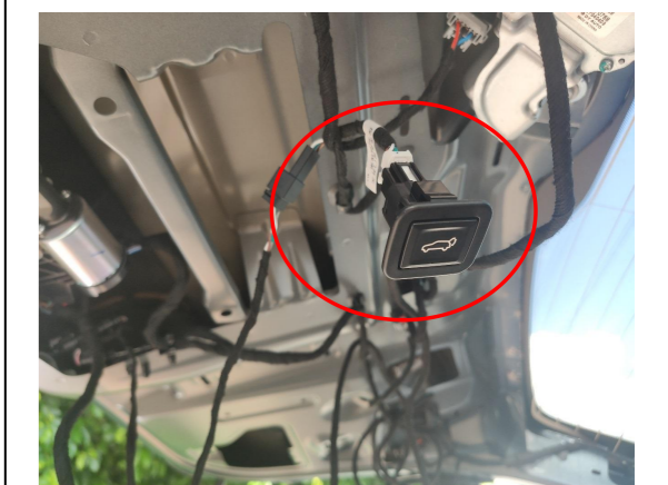
11. Connect the lock signal harness to the added tailgate switch.
