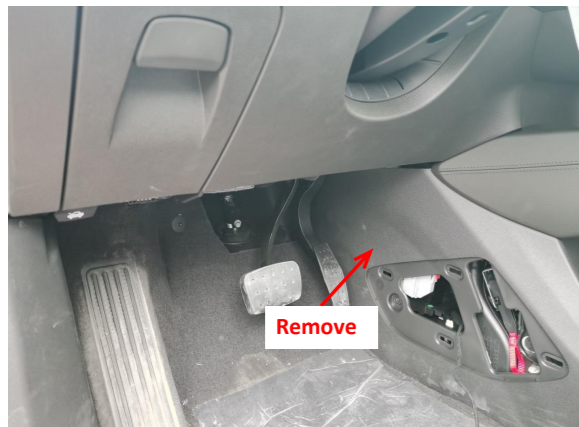
2. Remove the trim panel on the right side of the driver's area.
