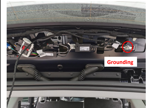
21. Ground at the indicated position of tailgate.
