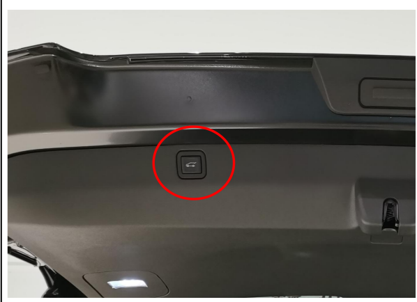
31. Reinstall all trim panel and fit the added tailgate switch in.
