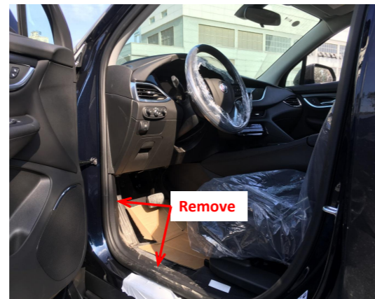
3. Remove the front left side trim panel and door sill panel.
