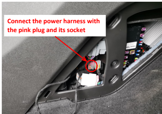
23. Connect the power harness to the indicated pink plug and its socket at the left side of the passenger seat.
