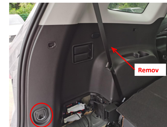
5. Remove the indicated trim panel from the left side of the trunk.
