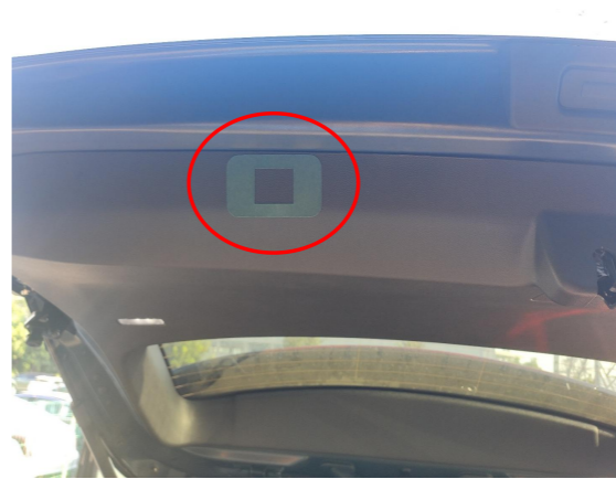
30. Stick the hole template to the indicated position and open a hole for the added tailgate switch.
