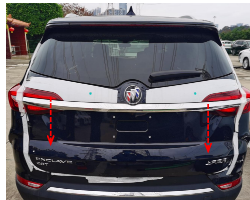
29. Press the added tailgate switch to open and close the tailgate once for initializing the system, and then test the functions of the electric tailgate.
