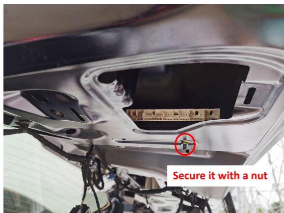
27. Secure the ECU bracket with a nut.
