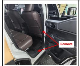
3. Remove the indicated rear right side door sill panel and B-pillar trim panel.
