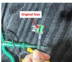
32. Move the fuse from the fuse box to the fuse tap.
