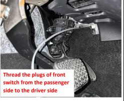
25. Thread the plugs of front switch from the passenger side to the driver side.
