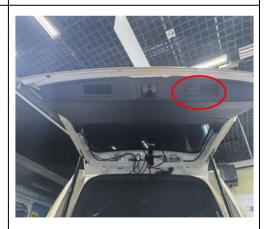
38. Remove the original tailgate handle, install the added tailgate switch and reinstall all the trim panels.
