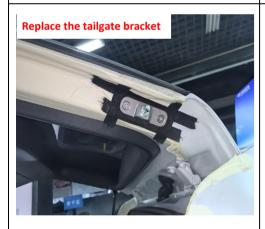
9. Replace the tailgate brackets on both sides of the tailgate.
