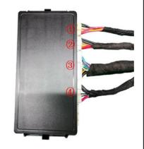
36. Insert the left and right strut wiring harnesses 12, lock signal harness (3), and power harness (4) into the ECU in sequence.
