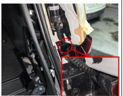
13. Reinstall the taillights and pay attention to the position of the strut wiring harness.
