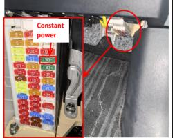
31. The fuse slot for power supply is indicated.
