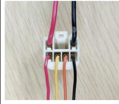
17. Insert the strut wiring harness terminals into the connector according to the diagram. (the connector is nserted on the ECU)
