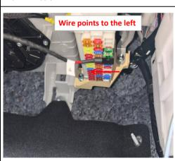
33. Plug the fuse tap into the fuse box and pay attention to the direction.
