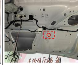
34. Secure the ECU bracket at the indicated position.
