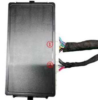
24. Insert the Lock signal harness ①, power harness ② into the ECU. Manually adjust the power latch to the locked state, press the original tailgate switch button and see whether the latch can be unlocked. If not, check whether the plugs are properly connected.
