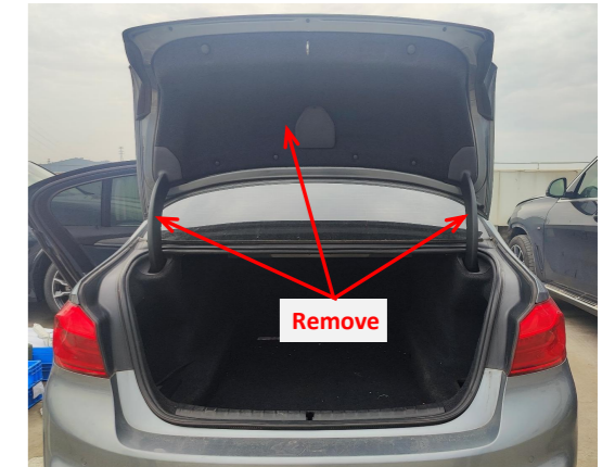
1. Remove the indicated trim panels from the tailgate and hinges.
