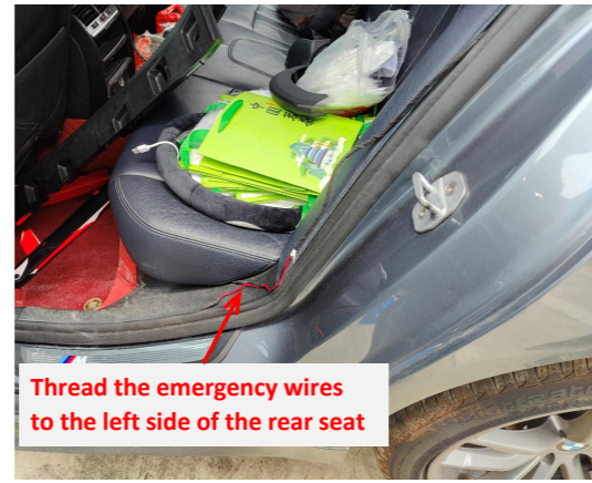
18. Thread the emergency wires to the left side of the rear seat and hide them in the trim panel.
