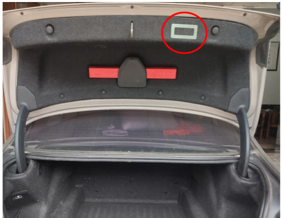
28. Stick the provided hole template to the indicated position and open a hole for the added tailgate switch.
