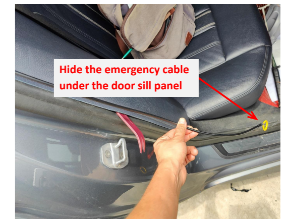
16. Thread the emergency cable to the right side of the rear seat and hide it under the door sill panel.
