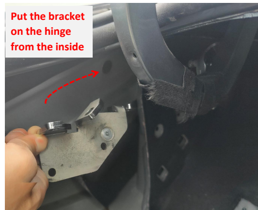
7. Install the left tailgate bracket on the left hinge.
