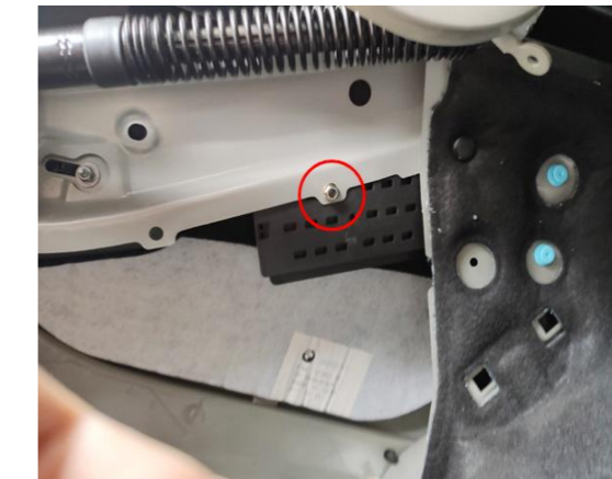
25. Install the ECU at the indicated position on the left side of the trunk.
