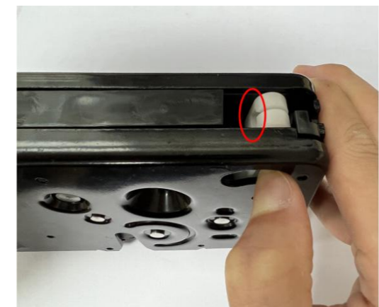
13. Unfasten the unlock arm of the power latch for installing the emergency cable.
