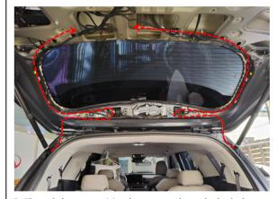
10. Thread the strut wiring harnesses through the holes on the tailgate and route the wiring harnesses as indicated.
