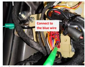
19-1. If you choose not to connect CAN signal, connect the orange wire of power harness to the indicated blue wire.
