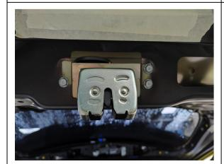
12. Remove the original latch and install the power latch.
