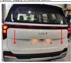
25. Press the added tailgate switch to close the tailgate once, the system completes initialization, and then test each function of the electric tailgate.
