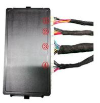
24.Insert the left and right strut wiring harnesses (1)(2), lock signal harness (3), and power harness (4) into the ECU in sequence.
