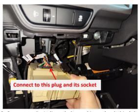
19. Connect to the indicated plug and its socket behind the fuse box.
