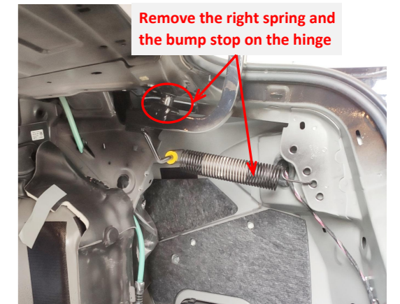
6. Remove the right spring and the bump stop on the right hinge.
