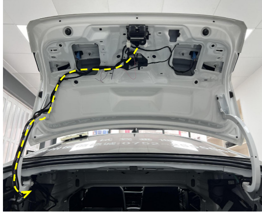
17. Route the lock signal harness to the left side of the trunk along with original wiring harnesses.
