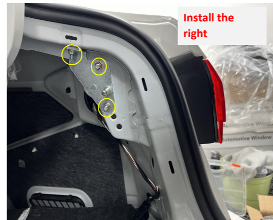
8. Install the right body bracket on the right side of the trunk.
