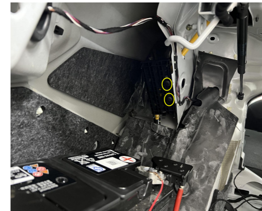
25. Secure the ECU bracket with nuts.
