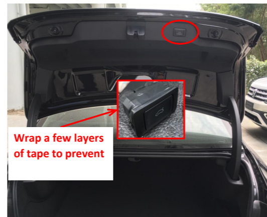
29. Reinstall all the trim panels and install the added tailgate switch.
