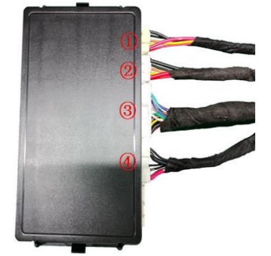
26. Insert the left and right strut wiring harnesses ① ②, lock signal harness ③, and power harness ④ into the ECU in sequence.
