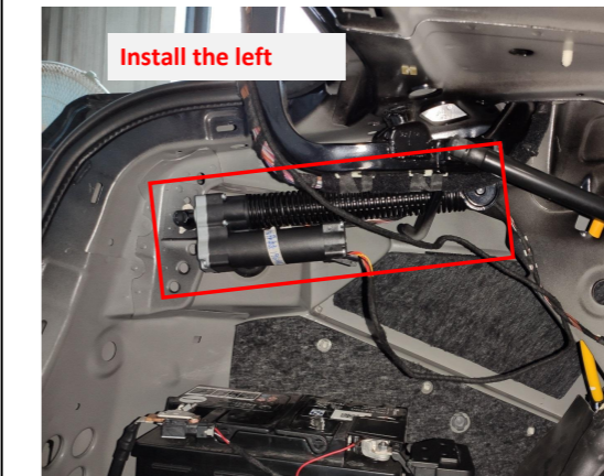
10. Install the left strut (L&R are marked as the first letter of the strut code).
