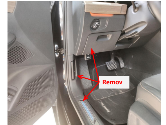
1. Remove the indicated driver's side trim panel door sill panel and storage box.
