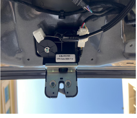
18. Install the power latch. (Manually adjust the latch to the locked state to prevent accidental closing during installation)
