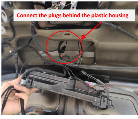
15. Connect the plugs of the lock signal harness to the original tailgate switch.
