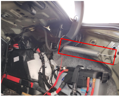
4. Remove the gas strut and the spring from the right side of the trunk.
