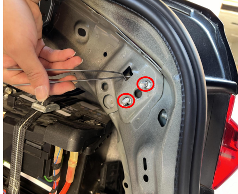
5. Install the right body bracket. Insert the bolts with handle from the indicated position into the car body.
