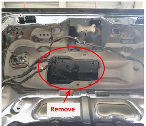
14. Remove the plastic housing from the tailgate.
