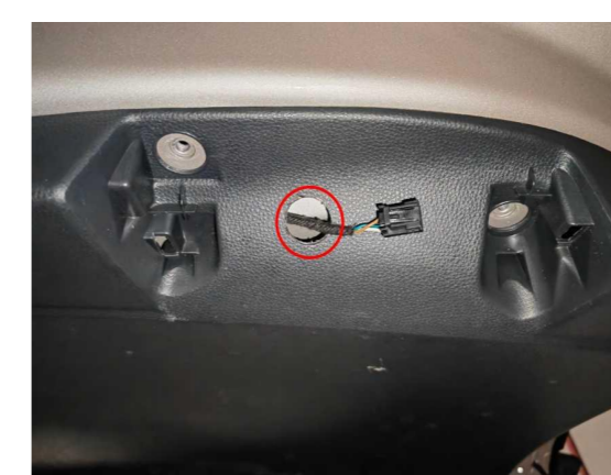
30. After opening the hole, pull out the plug of the tailgate switch.
