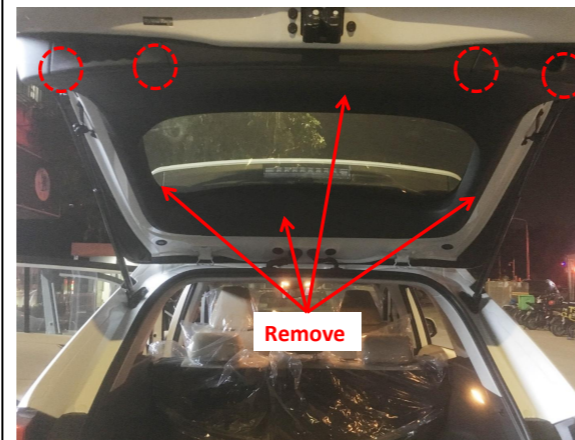
4. Remove the tailgate trim panels (there are screws in the circles).
