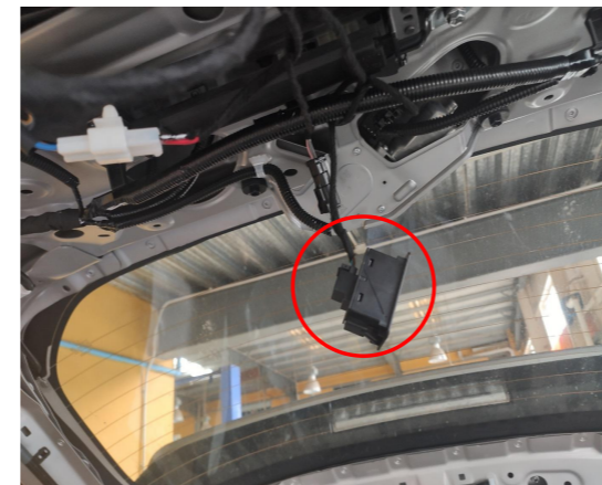
9. Install the added tailgate switch (the switch shown above is for test, and the actual switch may be different).
