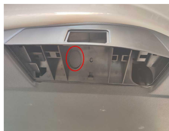
29. Fit the trim panel of our tailgate switch in (do not install the screw) and mark the indicated position for hole opening.
