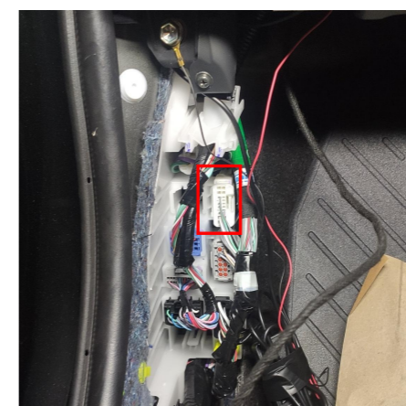
20. Connect the power harness to the signal plug and its mounting bracket.
