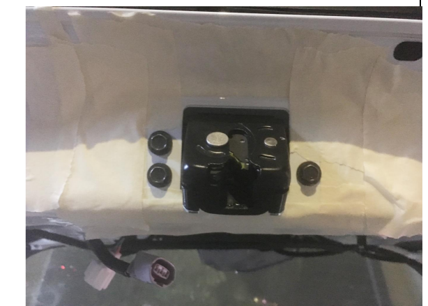
6. Remove the original latch and install our power latch.
