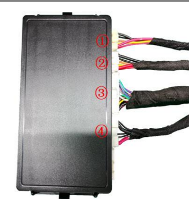
26. Insert the strut wiring harnesses ① ②, lock signal harness ③, and power harness ④ into the ECU in sequence and then mount the ECU on its bracket.
