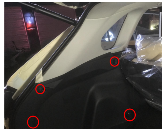
3. Remove the trim panel on the left side of the trunk (there are screws in the circles).
