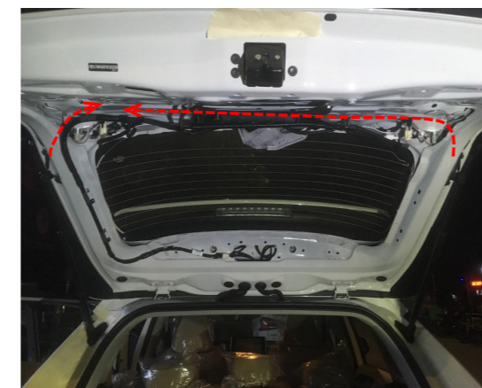
14. Thread the strut wiring harnesses through the original car holes and route them as shown above.
