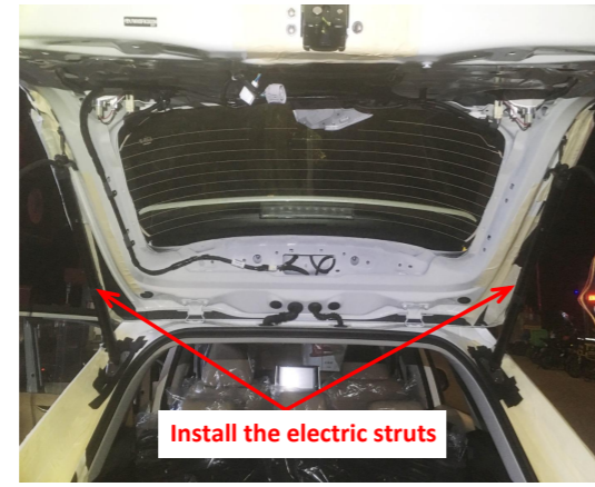
13. Install the electric struts, L on the left and R on the right (the first letter of the strut code).
