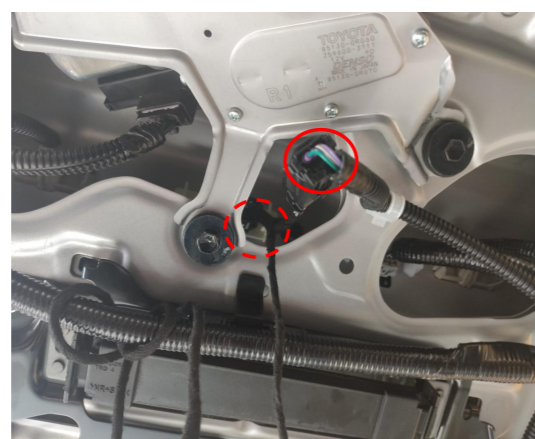
8. Connect the lock signal harness to the plugs of the original tailgate switch.
