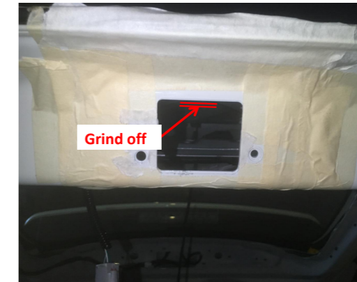
5. Remove the original latch and install the power latch. If the mounting hole interferes with the latch, grind off the upper outer frame for installation.
