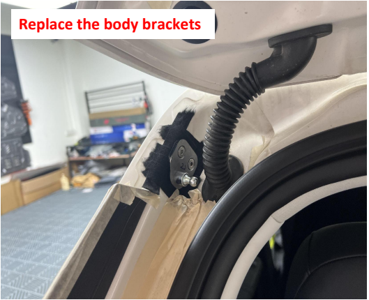
6. Replace the left and right body brackets.
