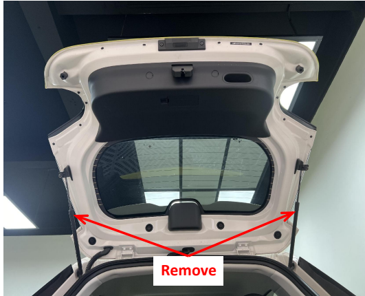
5. Remove the original gas struts.
