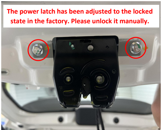
13. Install the power latch.
