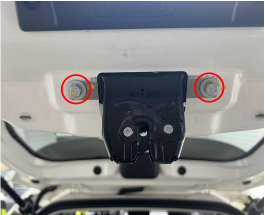
11. Remove the housing of the original latch and then remove the latch.
