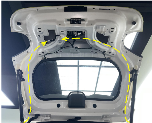
10. Route the strut wiring harness as indicated.
