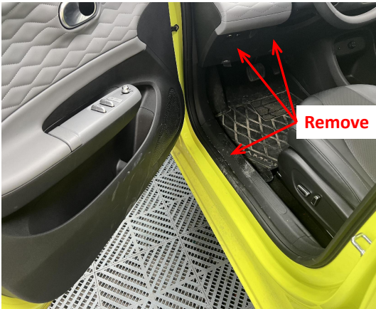
1. Remove the storage box trim panel and the front left side door sill panel.
