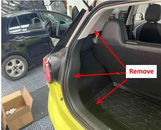
3. Remove the trim panels on the left side of the trunk and the trunk floor mat.
