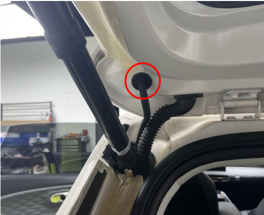
9. Thread the strut wiring harness through the indicated hole into the tailgate, the same on both sides.
