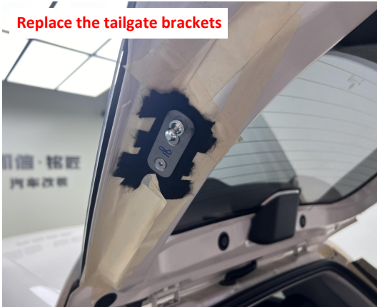
7. Replace the left and right tailgate brackets.
