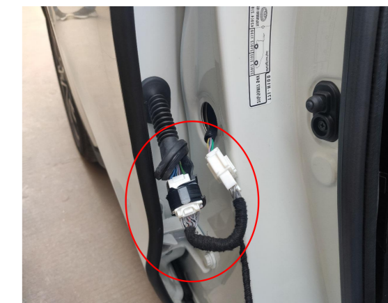
21. Connect the plugs of the power harness to the indicated plugs on the rear right side B-pillar.
