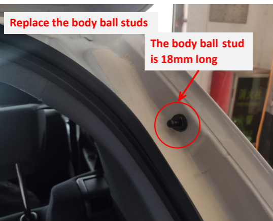
7. Replace the left and right body ball studs.
