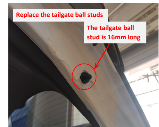
8. Replace the left and right tailgate ball studs.
