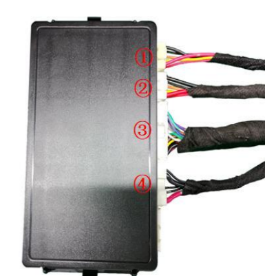
26. Insert the strut wiring harnesses ① ②, lock signal harness ③, and power harness ④ into the ECU in sequence and mount the ECU onto its bracket.
