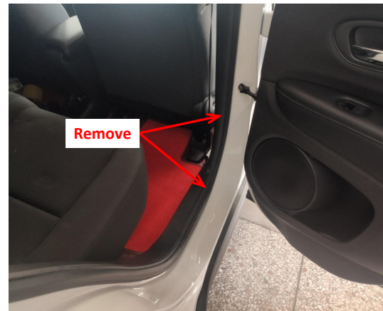
2. Remove the rear right door sill panel and B-pillar trim panel.
