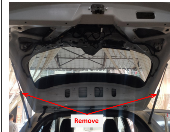
5. Remove the original gas struts.
