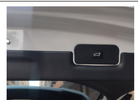
28. Reinstall all trim panels and fit the added tailgate switch in.
