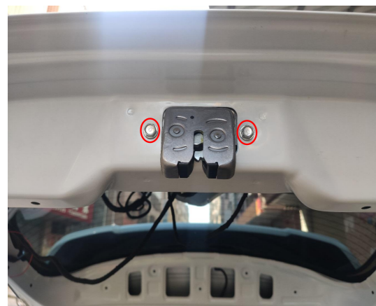
12. Remove the original latch and install our power latch.
