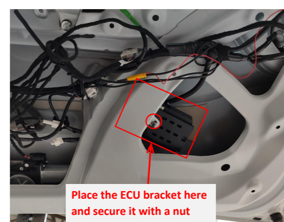
25. Place the ECU bracket at the indicated position and secure it with a nut.
