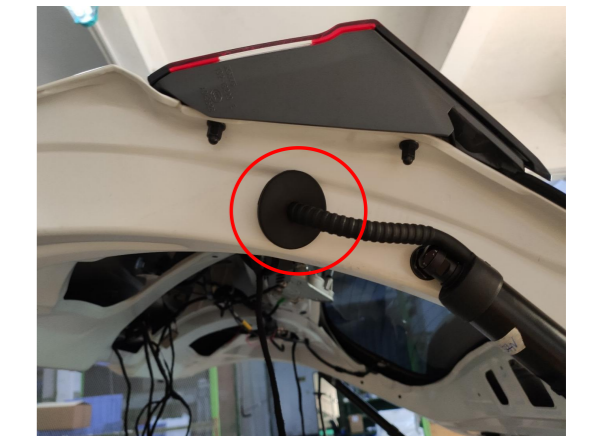
11. Thread the strut wiring harnesses through the holes and then plug the holes with hole plugs.
