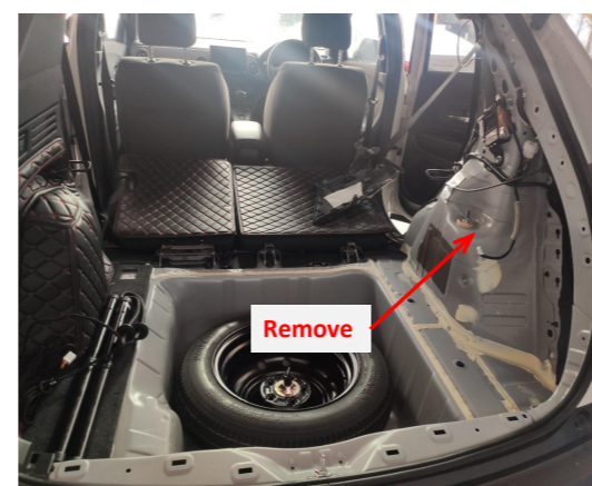
4. Take out the trunk floor mat and foam storage box. Remove the trim panel on the right side of the trunk.
