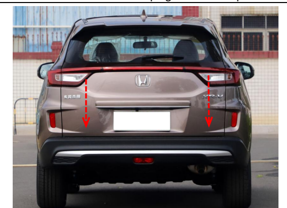
27. Press the added tailgate switch button to close the tailgate once for initializing the system and then test each function of the electric tailgate.
