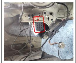
29. Secure the ECU at the indicated position with a nut.
