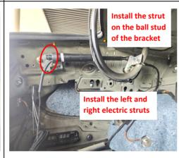
11. Install the left and right electric struts on the ball stud of the bracket (not the original car ball stud).
