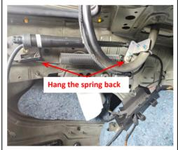
12. Hang the left springs back. Hang the long end at the body bracket and hang the short end between the two
