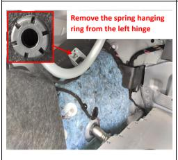
3. Remove the spring hanging ring from the left hinge.
