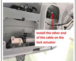
to ensure the latch can be unlocked)
