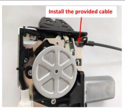
16. Install the provided cable on the power latch.
