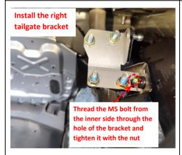
9. Install the right tailgate bracket: thread the M5 bolt through the bracket hole from the inner side and tighten t with the nut
