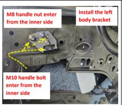
to secure the bracket first and then thread the M10
