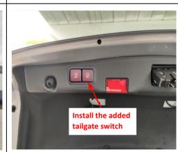
38. Reinstall all trim panels and install the added tailgate switch.
