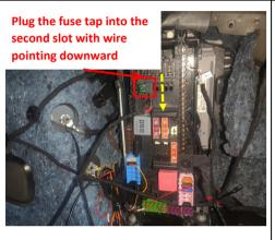
27. Plug the fuse tap into the second slot and pay attention to the direction.
