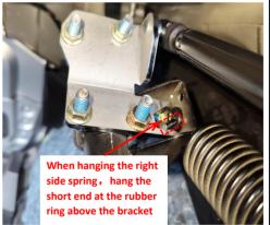
13. Hang the right springs back. Hang the long end of the spring at the body bracket and hang the short at the original spring hanging ring.
