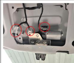
18. Install the emergency cable. (use the mechanical key 19. Connect the plugs of the lock signal harness to the plugs of the power latch.
