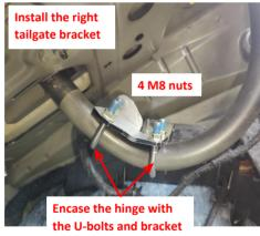
10. Encase the hinge with the U-bolt and bracket and tighten the bolt with the M8 nut.
