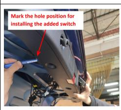
33. Fasten the trim panel to be pierced, align it with the hole of the sheet metal, and mark the hole position with 34. Mark it. a pen.
