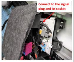
25. Connect to the signal plug behind the fuse box on the right side of the trunk.
