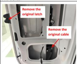
15. Remove the original latch and cable.
