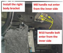
1. Install the left body bracket: thread the M8 handle nut 5. Install the right body bracket: thread the M8 handle nut to secure the bracket first and then thread the M10
