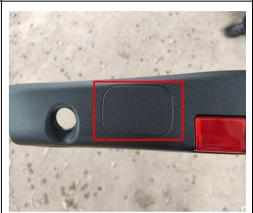
32. Open a hole at the indicated position for installing the added switch.
