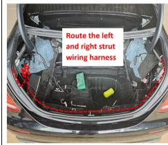
14. Route the left and right strut wiring harnesses to the left side of the trunk.
