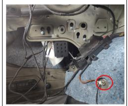
24. Ground at the indicated position on the left side of the trunk.
