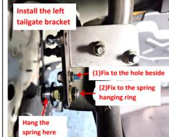
. Install the left tailgate bracket: remove the M10 nut, thread the M10 bolt through the spring hanging ring and en screw the nut and fasten the M6 bolt.
