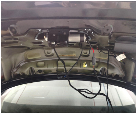
9. Install the power latch with original screws and confirm that the latch has been locked.
