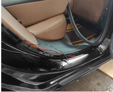
10. Route the two emergency wires along the right hinge to the right side of the rear seat and hide them under the door sill panel.
