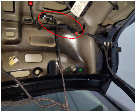
8. Connect the plugs of the lock signal harness to the original tailgate switch.
