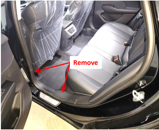
2. Remove the rear left door sill panels.
