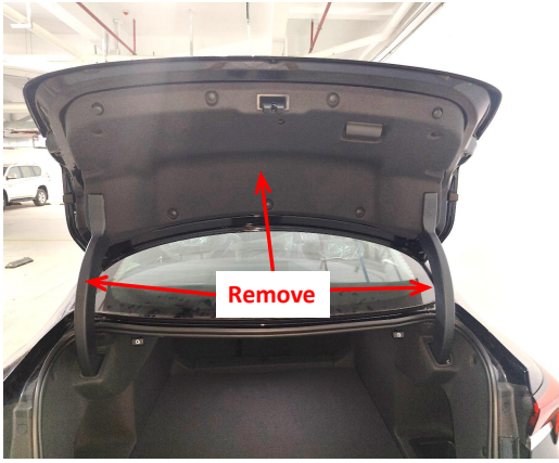
4. Remove the indicated trim panels from the tailgate and hinges.
