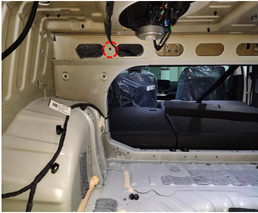
14. The indicated hole is the center of the body bracket.
