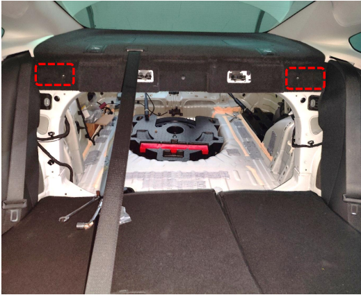
16. Remove the fasteners from the trim panel that connects to the trunk, lift up the corners on both sides to fasten the
