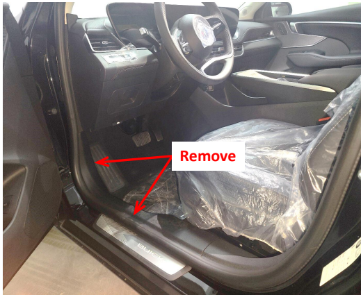
1. Remove the front left door sill panels.
