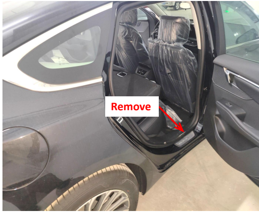
3. Remove the rear right door sill panel.
