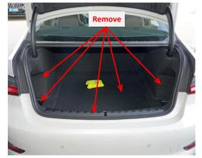
2. Remove the indicated trim panels and floor mat from the B. Remove the left and right springs and install the right trunk. body bracket at the indicated hole.
