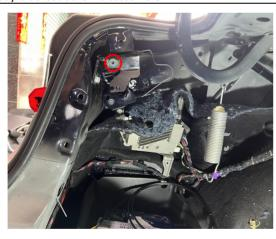
8. Screw the countersunk screw into the nut.
