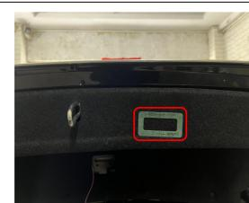
33. Stick the provided hole template to the indicated position and open a hole for the added tailgate switch.
