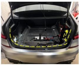
12. Install the electric struts, L on the left, R on the right (the 13. Route the strut wiring harnesses to the right side of the trunk along with original wiring harness.
