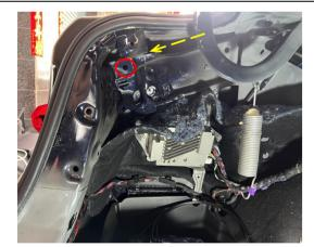
7. Thread the M10 nut with a handle to the indicated position to install the left body bracket.
