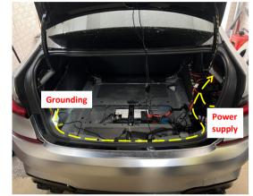
22. Route the power harness to the right side of the trunk along original wires.
