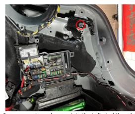
Screw a countersunk screw into the indicated threaded nole
