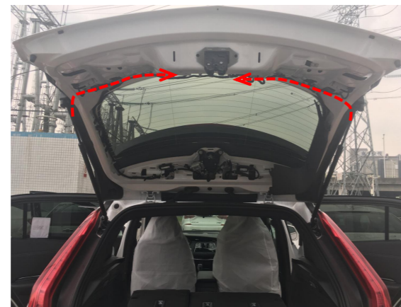
13. Route the strut wiring harnesses as indicated above.
