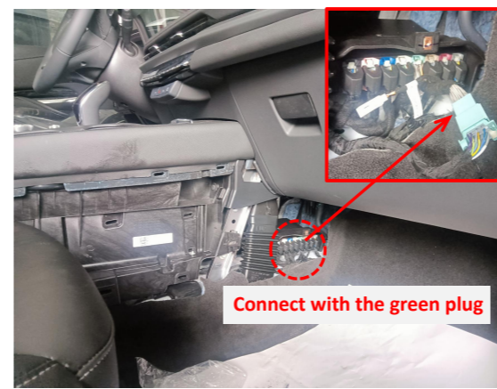
24. Connect the signal plug to the indicated green plug.
