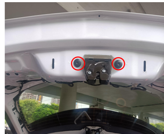
14. Remove the original latch.
