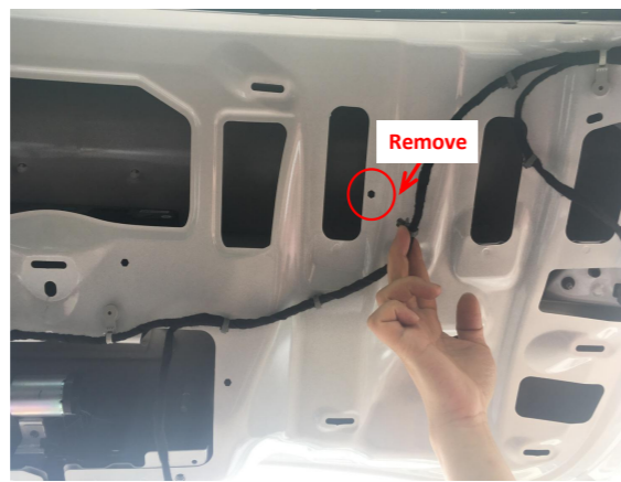
28. Remove the indicated wire clip.
