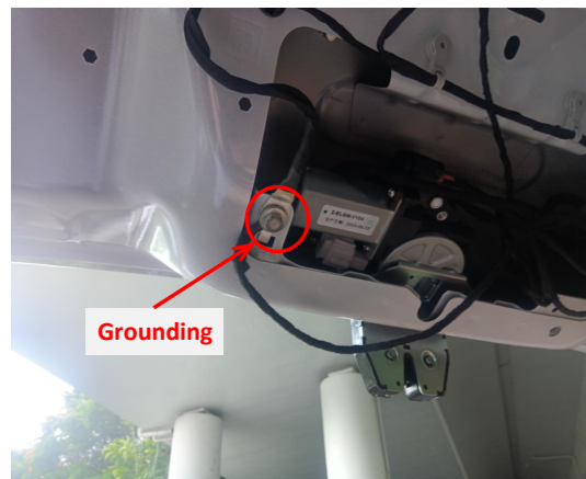
22. Ground at the indicated position
