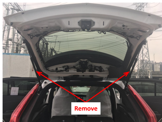
7. Remove the original gas struts.
