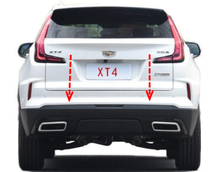
31. Press the added tailgate switch button to open and close the tailgate once, the system will complete initialization, and then test the each function of the electric tailgate.
