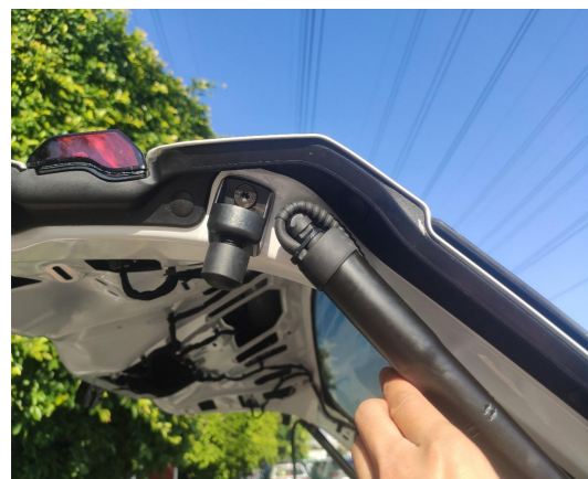
12. Tie the rubber tube as shown above.
