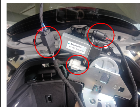
15. Connect the lock signal harness to the plugs of the power latch.
