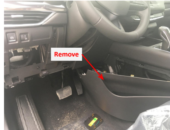
3. Remove the indicated trim panel.
