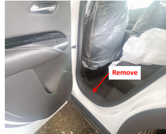
4. Remove the rear left door sill panel.
