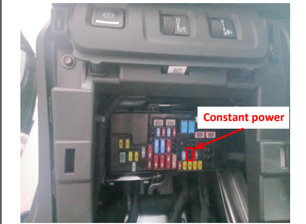
26. The fuse slot for power supply is indicated above.
