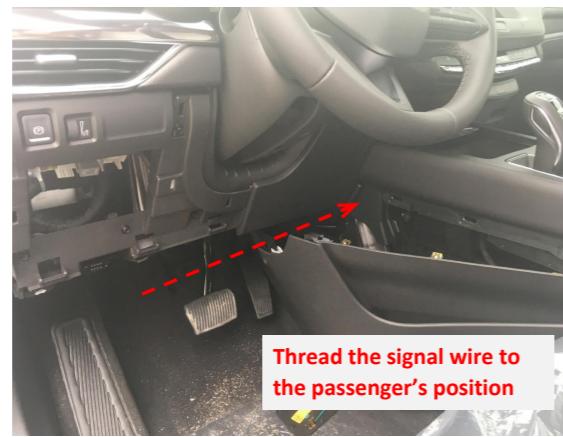
23. Thread the signal plug of the power harness to the front passenger's area.
