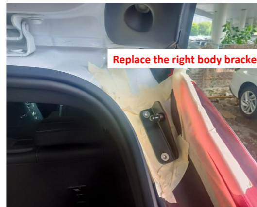
9. Replace the right body bracket.
