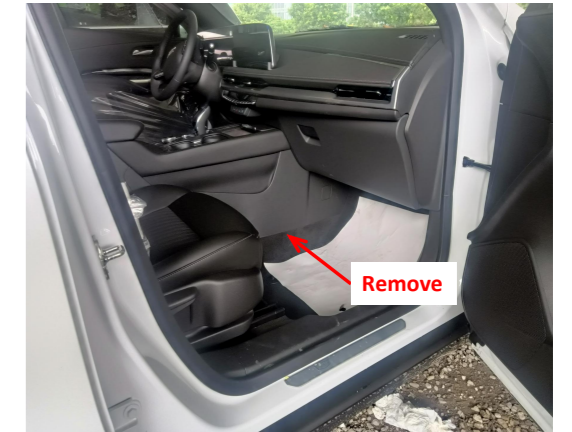
1. Remove the indicated trim panel.
