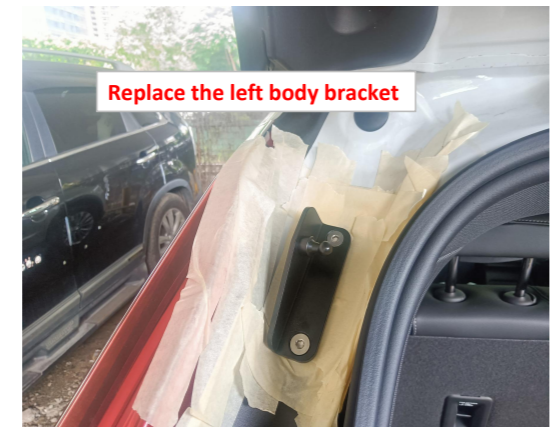
8. Replace the left body bracket.
