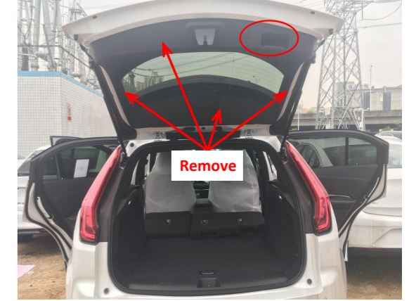
6. Remove the indicated trim panels from the tailgate.
