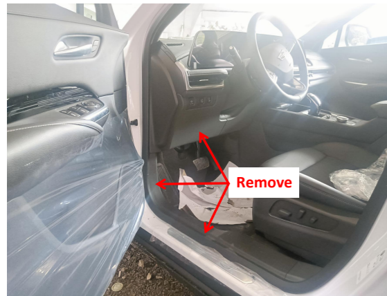
2. Remove the indicated door sill panels and the trim panel of fuse box.
