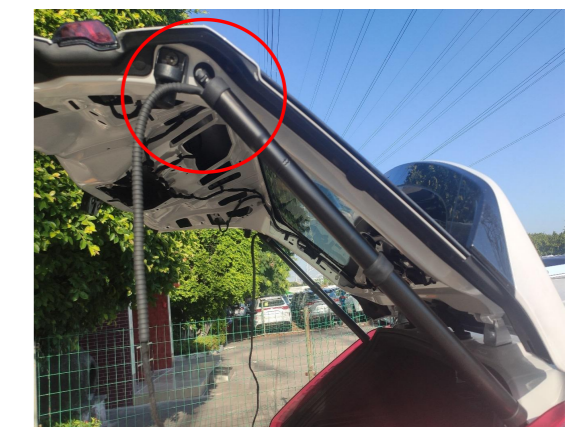
11. Install the electric struts, L on the left and R on the right (the first letter of the strut code).
