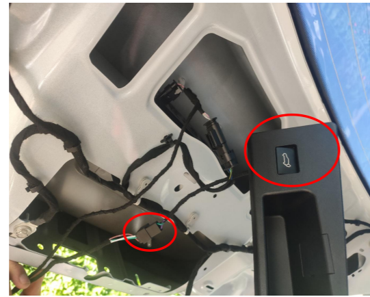
18. Connect the plug of the lock signal harness to the added tailgate switch.
