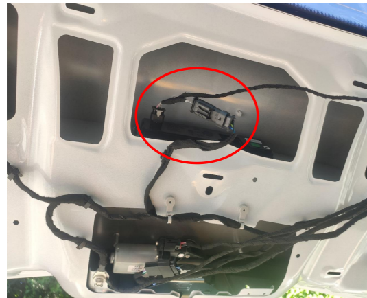
17. Connect the plugs of the lock signal harness to the original tailgate switch.
