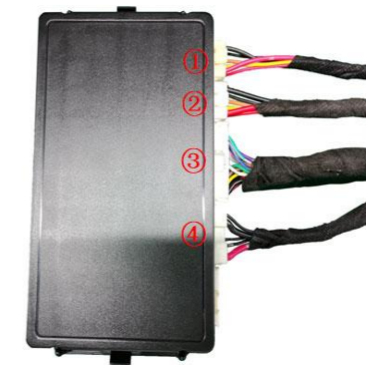
30. Insert the left and right strut wiring harnesses ①②, lock signal harness ③, and power harness ④ into the ECU in sequence.
