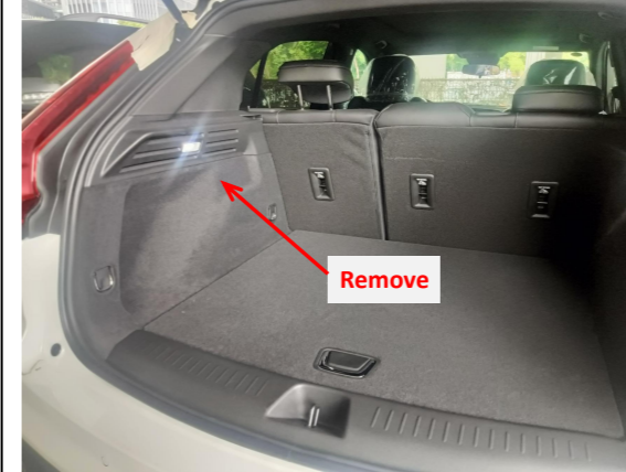
5. Remove the indicated panel to allow wiring harnesses to pass through.
