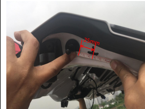
10. Drill a hole at the indicated location on both sides with a \phi 21\text{mm} drill bit to allow the wiring harnesses to pass through.
