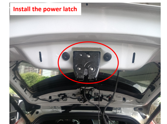
16. Install the power latch.
