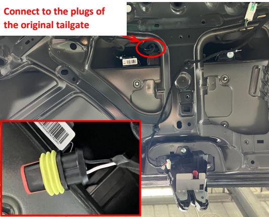
14. Connect the lock signal harness to the plugs of the original tailgate switch.
