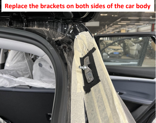
6. Replace the brackets on both sides of the car body and pay attention to the direction of the ball studs.
