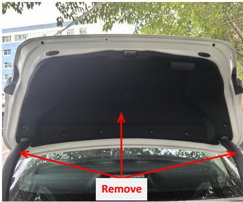
3. Remove the indicated tailgate trim panels.
