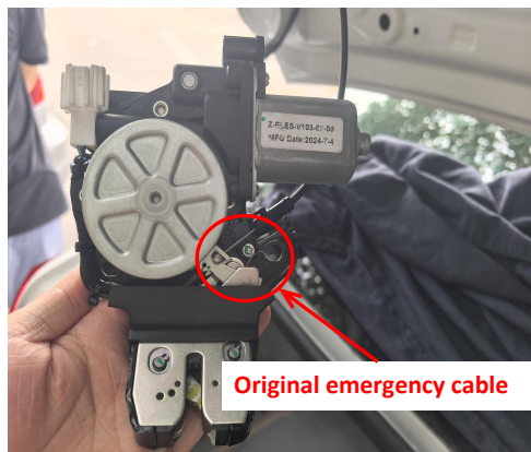
20. Install the original emergency cable on the inner fastener of our power latch.
