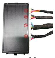
25. Insert the strut wiring harnesses (1)(2), lock signal harness (3), and power harness (4) into the ECU in sequence.
