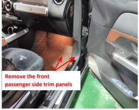
2. Remove the trim panels on the right side of the passenger 3. Lift the floor mat of the passenger seat and find out the
