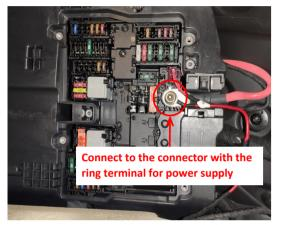
22. Connect to the indicated connector with the ring terminal for power supply.
