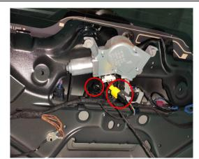
16. Connect the lock signal harness to the plugs of the original tailgate switch and the added tailgate switch.
