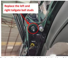
8. Replace the ball studs on the left and right sides of the tailgate.
