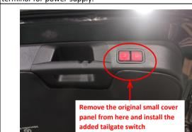
27. Install all trim panels back and install the added tailgate switch. Check whether the buttons can bounce back normally. If there is any interference, use a knife to scrape the interfering part.)
