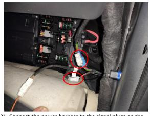
21. Connect the power harness to the signal plugs on the right side of the passenger seat.
