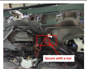
23. Place a bolt at the ECU bracket and mount the ECU onto 24. Install the ECU at the indicated position and secure it with a nut.
