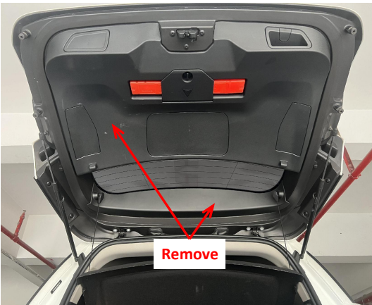
4. Remove the tailgate trim panels.
