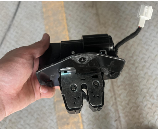
14. Fit the power latch onto the sheet metal of original latch.
