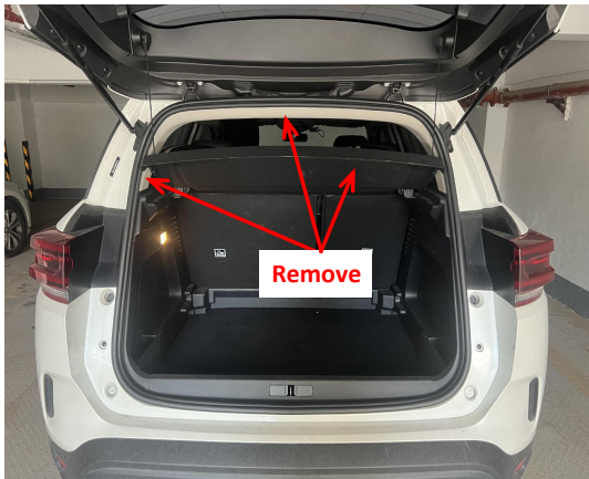
3. Remove the indicated trim panels and sun visor.
