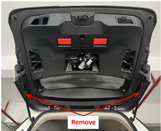
6. Remove the original gas struts.
