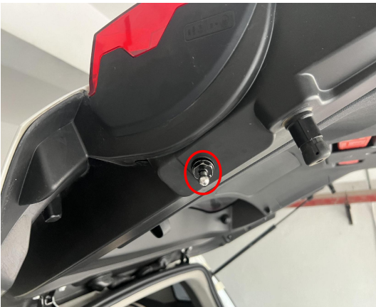
9. Replace the ball studs on both sides of the tailgate.
