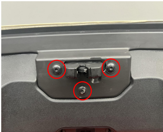
13. Remove the original latch.
