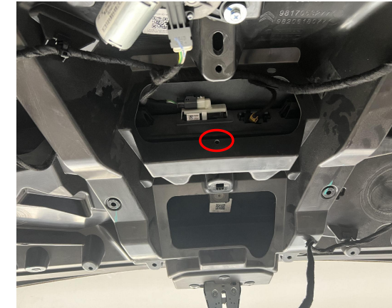
25. Drill a hole at the indicated position with a 6mm drill bit.
