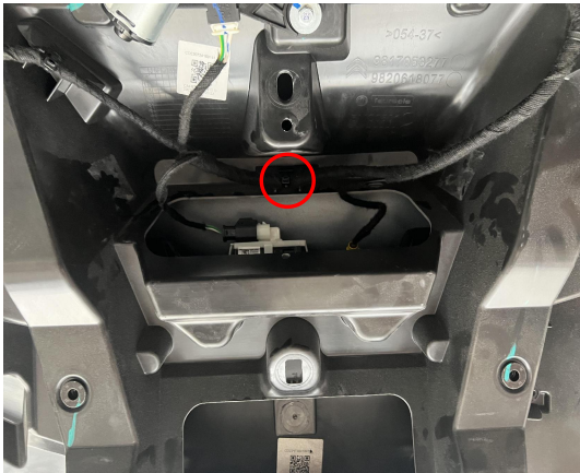
27. Remove the indicated cable clip.
