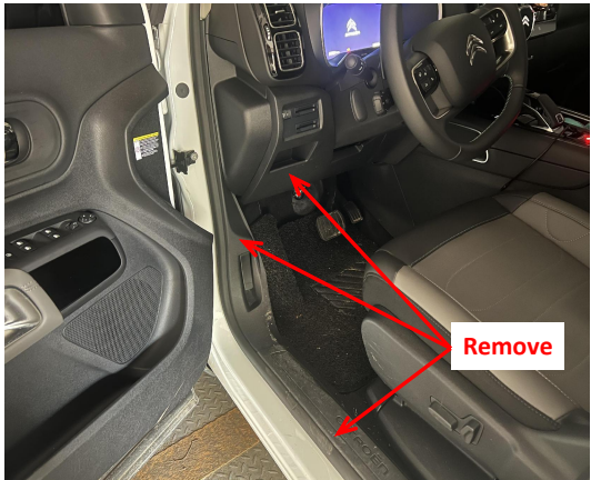
1. Remove the indicated driver's side trim panels.
