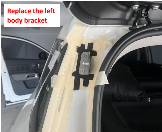
7. Replace the left body bracket.
