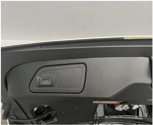
32. Install the added tailgate switch and reinstall all the trim panels.
