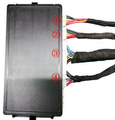
27. Insert the strut wiring harnesses ①②, lock signal harness ③, and power harness ④ into the ECU in sequence, and then mount the ECU on its bracket.
