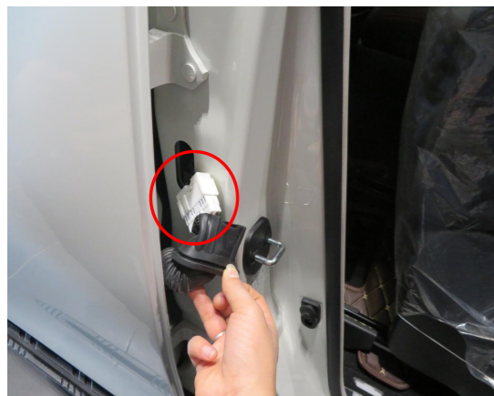
22. Connect the plugs of the power harness to the B-pillar signal plugs.
