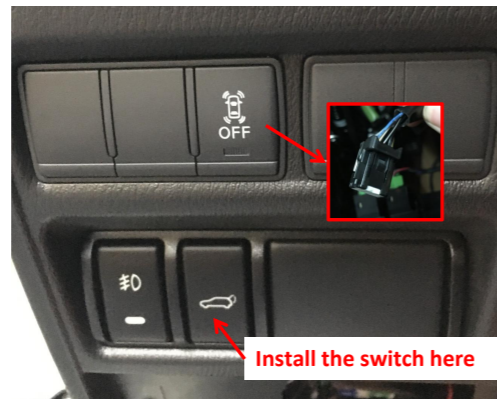
23. Install the switch at the indicated position. The small illustration shows the connection between the signal connector of backlight and our wiring harness connector.
