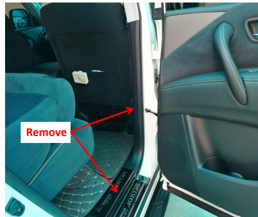
2. Remove the rear right side door sill trim panel and B-pillar trim panel.
