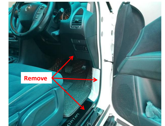
1. Remove the front right side trim panel, door sill trim panel and the exterior trim panel of fuse box.
