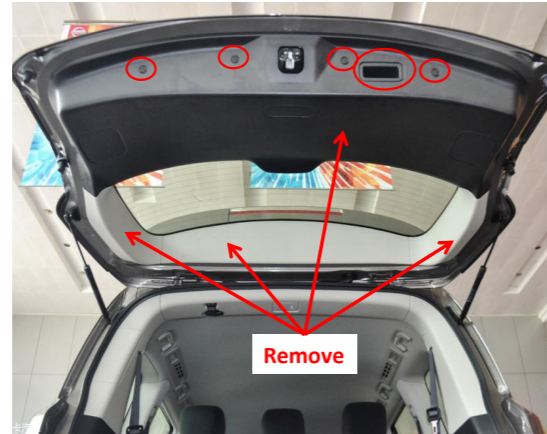
3. Remove the tailgate trim panels.
