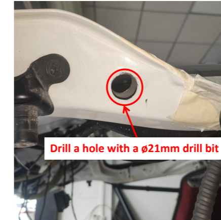
15. Use a ø21mm drill bit to drill a hole through two layers at the indicated position. Both sides are the same.
