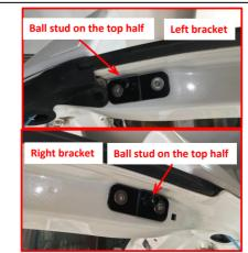
15. Replace the left and right tailgate brackets (the ball studs are on the top half and near the spoiler).
