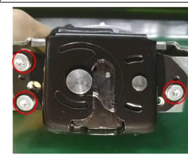
8. Remove the screws from the power latch.
