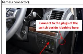
27. Remove the blank button from the switch panel and install the added front switch.
