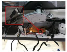
'. Connect the plugs of lock signal harness with the original tailgate switch (because the original tailgate switch plugs of the 2016 and 2018 models are different, two pairs of plugs are reserved, and choose the correct one pair according to the year).
