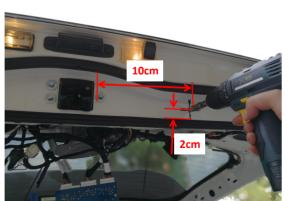
tailgate switch using a \$14mm drill bit.
