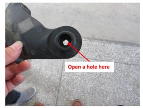
18. Open a hole at the indicated position of the rubber pads | 19. Remove the screw from the hole and thread the strut (as long as the plugs of strut wiring harness can fit through). wiring harness through the hole.
