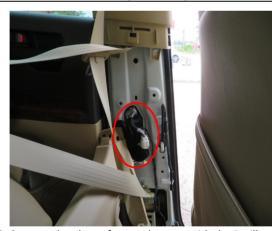
28. Connect the plugs of power harness with the B-pillar signal plugs.
