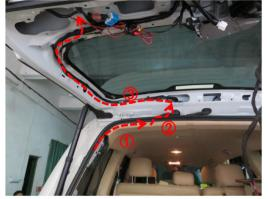
22. Thread the power harness to the left side of tailgate (do not connect plugs before inserting terminals into wiring
