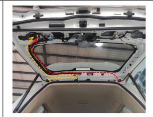
20. Route the strut wiring harnesses as indicated.
