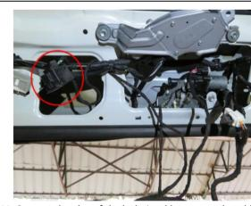
11. Connect the plug of the lock signal harness to the added tailgate switch.
