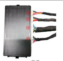
30. Insert the strut wiring harnesses (1)(2), lock signal harness (3), and power harness (4) into the ECU in sequence, and mount the ECU on its bracket.
