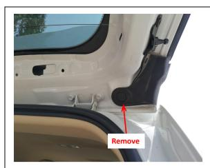
17. Remove left and right tailgate rubber pads.
