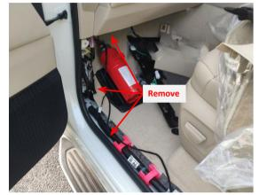
2. Remove the front left side trim panels, door sill panel and 3. Remove the rear left door sill panel and B-pillar trim storage box.
