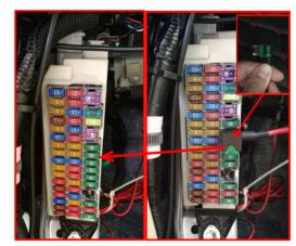
29. Move the indicated fuse (sixth in the rightmost column), to the fuse tap and then plug the fuse tap into the fuse box.
