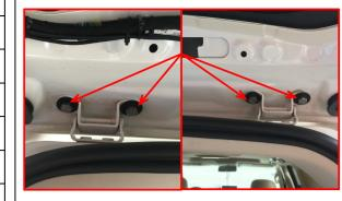
1. Add the reinforcing washers to the hinges and secure them with provided screws.
