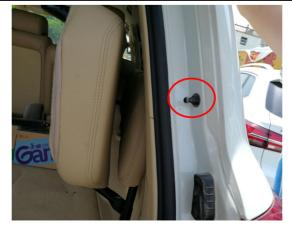
14. Replace the left and right body ball studs.
