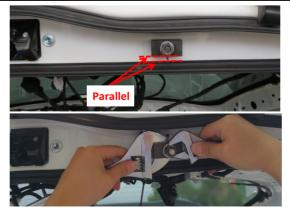
4.Install the hole opener (make sure its edge is parallel to the ower edge of the tailgate) and open the hole (one wrench holds the hole opener and the other wrench turns the nut).
