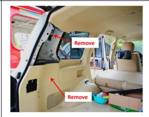
5. Remove the trim panels on the left side of the trunk.
