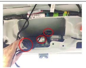
10. Connect the plugs of the lock signal harness to the power latch.
