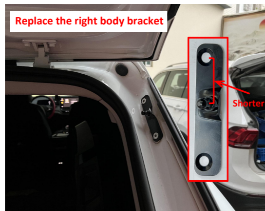
8. Replace the bracket on the right side of the car body making sure the ball stud is closer to the top of the bracket.
