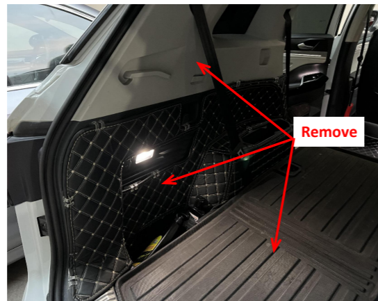
3. Remove the trunk floor mat and the trim panels on the left side.
