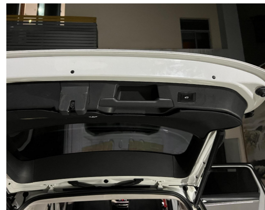
27. Install the added tailgate switch and reinstall all trim panels.
