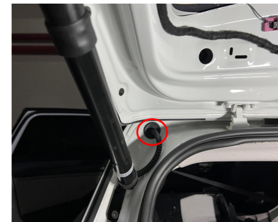
10. Thread the strut wiring harness through the indicated hole into tailgate.
