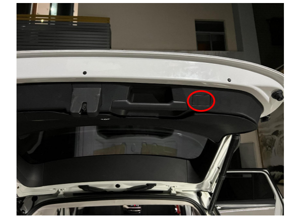
26. Remove the indicated small panel for installing the added tailgate switch.
