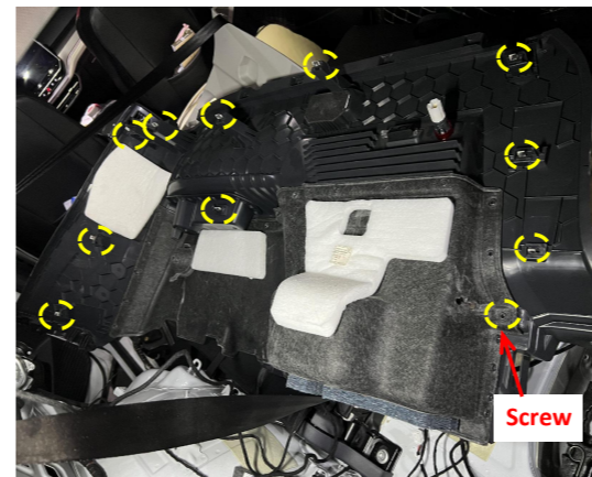
4. Pay attention to the locations of the screws and fasteners.
