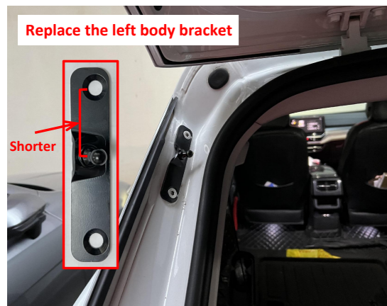
7. Replace the bracket on the left side of the car body making sure the ball stud is closer to the top of the bracket.
