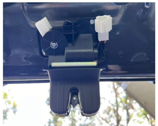
13. Install our power latch and cover the latch with original plastic casing.
