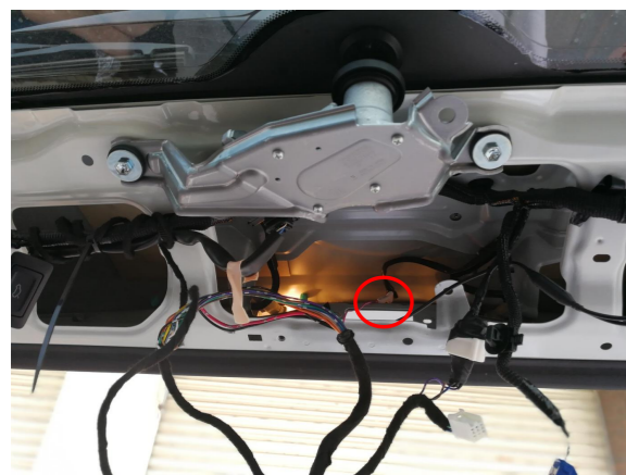
7. Connect the plugs of the lock signal harness to the original tailgate switch
