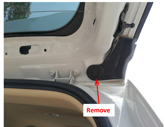
16. Remove left and right tailgate rubber pads.
