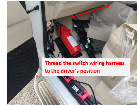
25. Thread the switch wiring harness to the driver's position.
