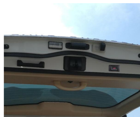
33. Install all the trim panels back and install the added tailgate switch.
