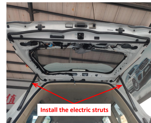
15. Install the electric struts, L on the left and R on the right (the first letter of the strut code).
