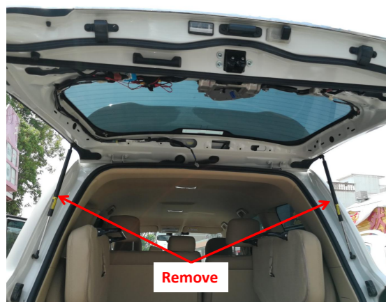
12. Remove the gas struts.
