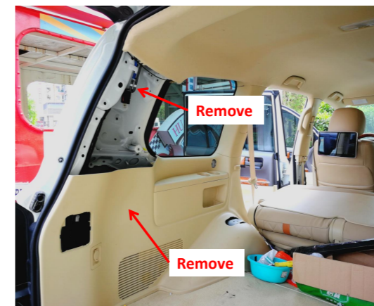
5. Remove the trim panels on the left side of the trunk.
