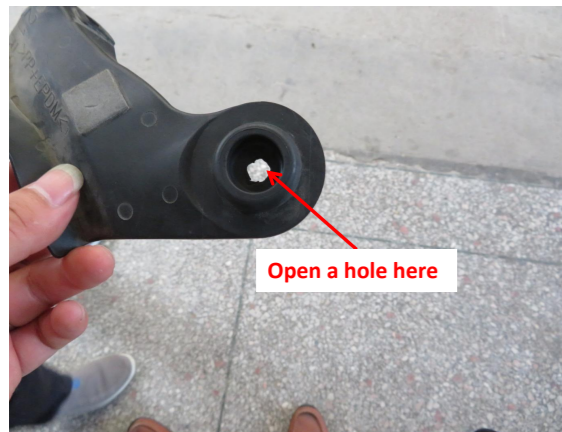
17. Open a hole at the indicated position of the rubber pads (as long as the plugs of strut wiring harness can fit through).
