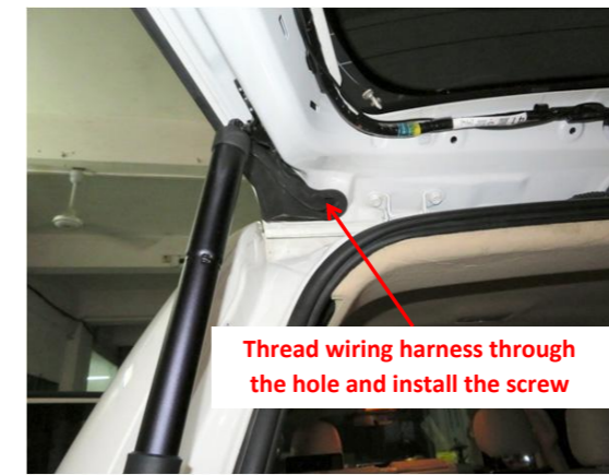
20. Reinstall the screw and plug the hole tightly. Both sides are the same.
