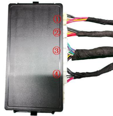
29. Insert the strut wiring harnesses ①②, lock signal harness ③, and power harness ④ into the ECU in sequence, and mount the ECU on its bracket.
