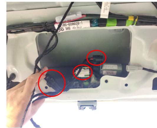
10. Connect the plugs of the lock signal harness to the added power latch.
