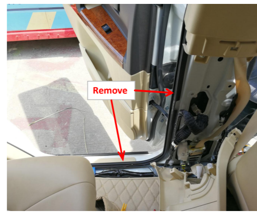
3. Remove the rear left door sill panel and B-pillar trim panel.
