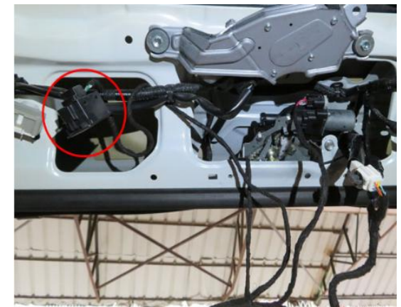
11. Connect the plug of the lock signal harness to the added tailgate switch.
