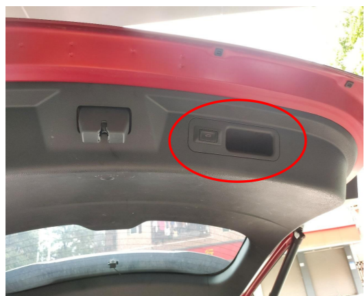
27. Reinstall all trim panels and install the added tailgate switch.
