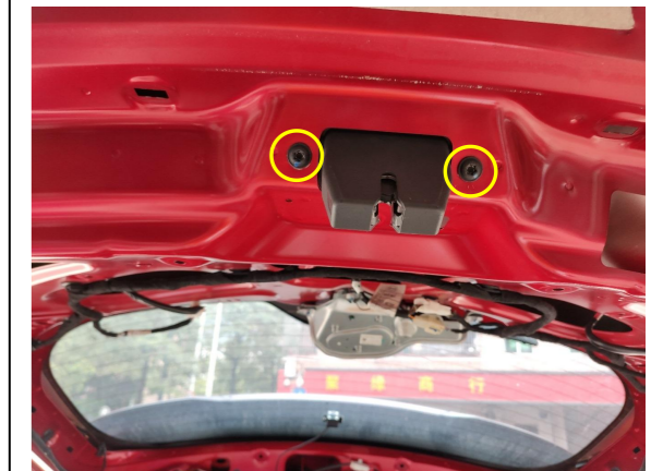
11. Remove the original latch.
