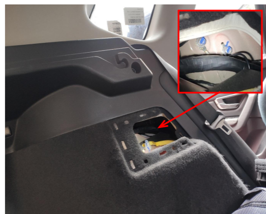
18. Ground at the left side of the trunk.
