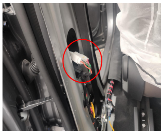
19. Connect power harness to the B-pillar plugs at rear left side B-pillar.
