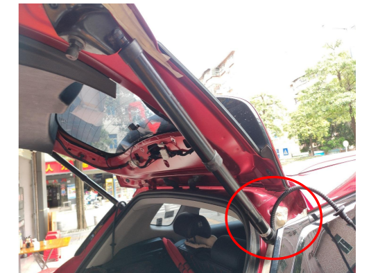
6. Install the electric struts, L on the left and R on the right (the first letter of the strut number), making sure the ends with wiring harnesses are on the vehicle body.
