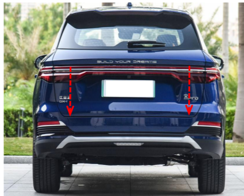
24. Press the added tailgate switch button to open and close the tailgate once for initializing the system, and then test each function of the electric tailgate.
