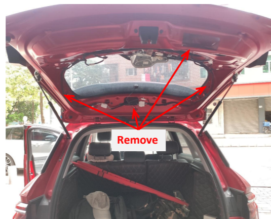
3. Remove the tailgate trim panels.
