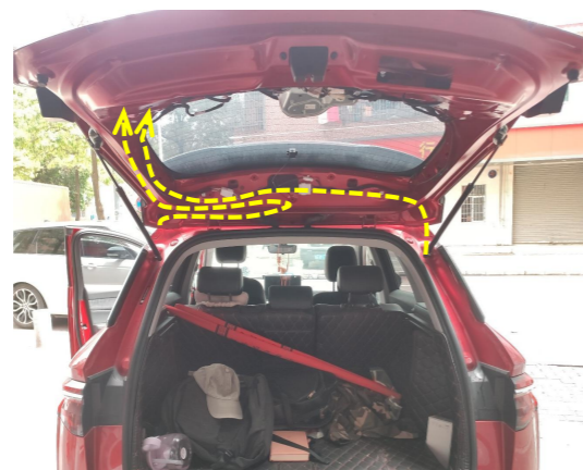
8. Route the strut wiring harness to the tailgate.
