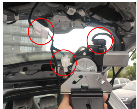
12. Connect the lock signal harness to the plugs of our power latch.
