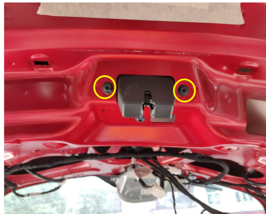
13. Install the power latch.
