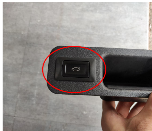
26. Fit the added tailgate switch in.
