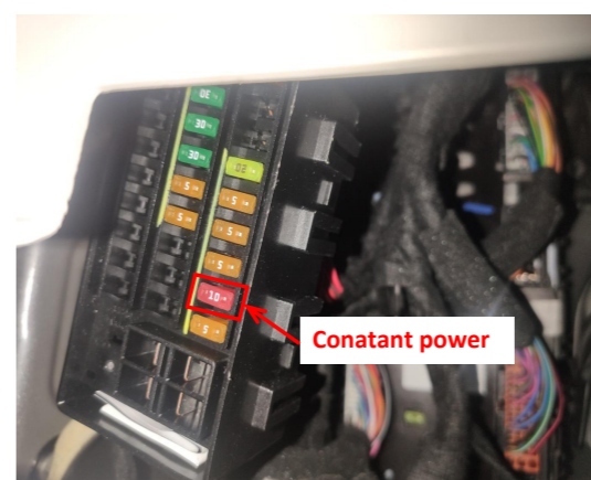
20. The fuse box is located behind the storage box and the fuse slot for power supply is indicated above.
