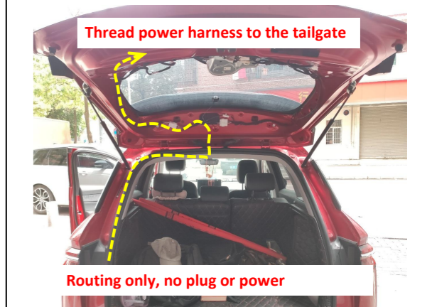
16. Thread the power harness to the tailgate (routing only, no plug or power connection).
