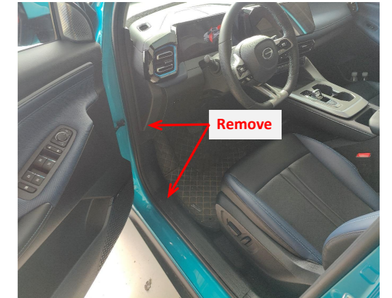
1. Remove the indicated driver's side trim panels.
