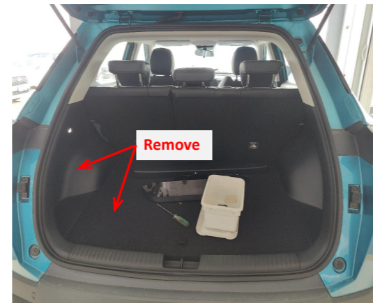
4. Remove the trunk floor mat and the trim panel on the left side.
