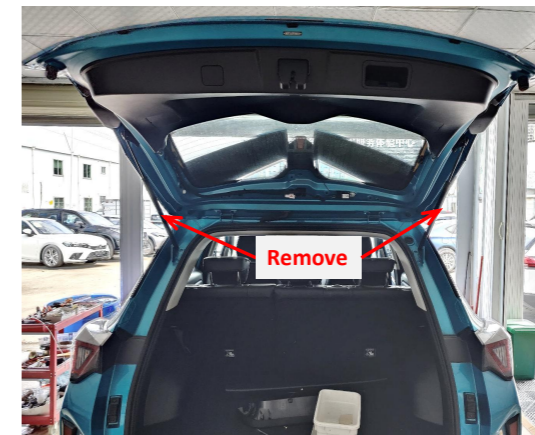
5. Remove the original gas struts.
