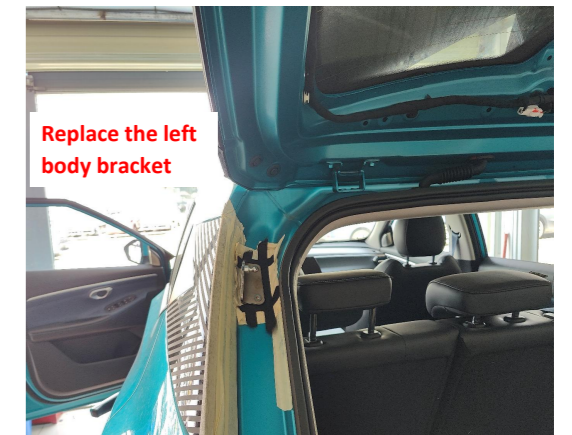
6. Replace the left body bracket.
