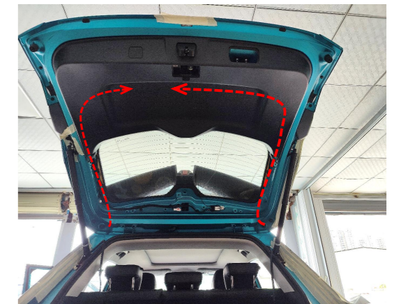
11. Route the left and right strut wiring harness to the tailgate as indicated.
