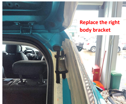
7. Replace the right body bracket.
