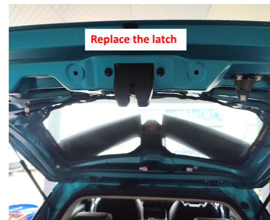
14. Remove the original latch and install the power latch.
