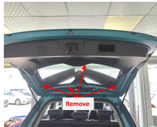
3. Remove the indicated tailgate trim panels.
