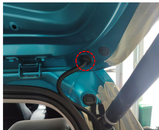
12. Plug the hole plug of the strut wiring harness into the indicated hole, the same on both sides.
