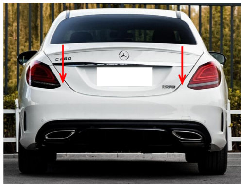
28. Manually close the tailgate until it touches the striker, then press the original tailgate switch button to open the tailgate. The system will complete initialization, and then test each function of the electric tailgate.
