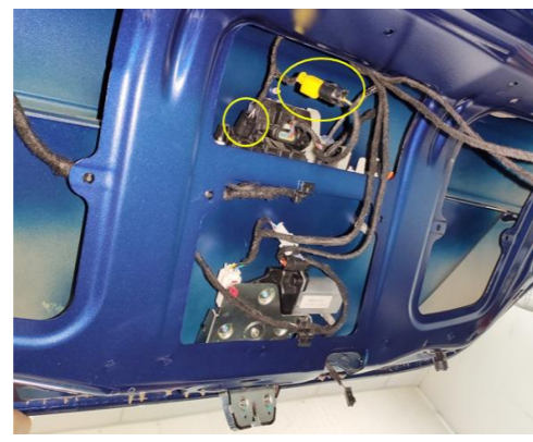
18. Connect the plugs of the lock signal harness to the plugs of the original tailgate switch and the added tailgate switch.
