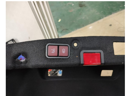
31. Open the hole and fit the added switch in. Check whether the buttons can bounce back normally when pressed and then reinstall all the trim panels
