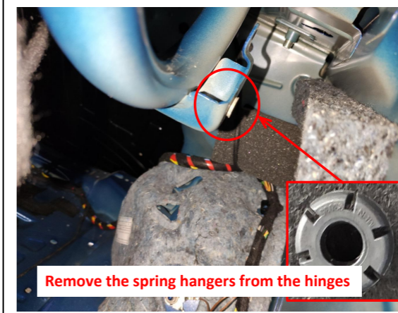
5. Remove the spring hangers from the left and right hinges.
