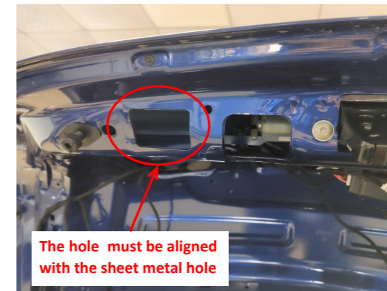
30. The hole of the added tailgate switch must be aligned with the sheet metal hole.
