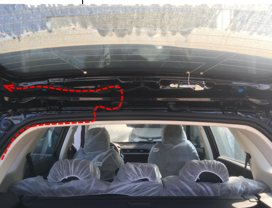
16. Route the power harness to the tailgate (no plug cord before inserting terminals into the connector).
