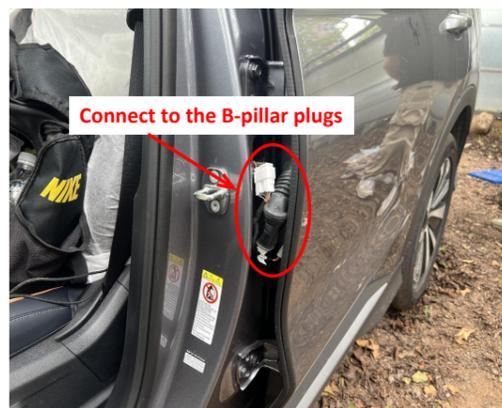
18. Connect to the B-pillar plugs at rear left B-pillar.
