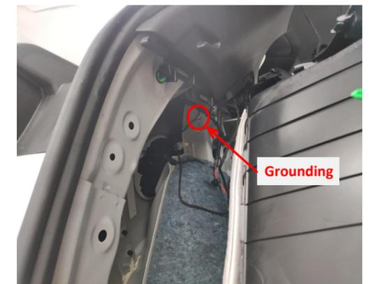
16. Ground at the indicated position on the left side of the trunk.
