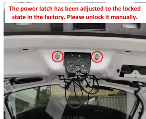
13. Install the power latch with provided screws.
