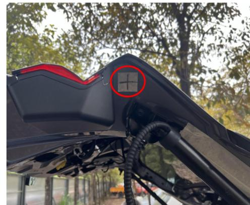
9. Open a hole at the indicated position on both sides to allow the wiring harnesses to pass through.
