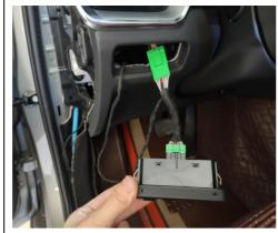
23. Connect the plugs to the front switch.(If there is a fuel tank flap button, then it does not need to connect to 24. Ground at the right side of the trunk. the front switch. e.g.: S90 T8)
