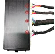
lock signal harness 3, and power harness 4 into the ECU in sequence and mount the into its bracket.
