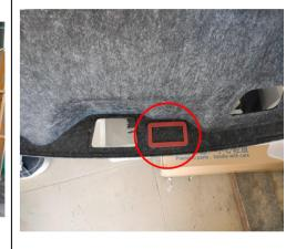
32. Stick the hole template to the indicated position and open a hole for the added tailgate switch.
