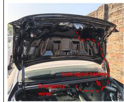
20. Route the lock signal harness along the original wires to prevent from being pulled during tailgate operation.
