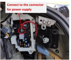
27. Connect to the fuse box on the right side of the trunk 28. Drill a hole at the indicated position and secure the
