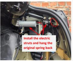
13. Install the electric struts, L on the left and R on the right (the first letter of the strut code) and hang the springs back.
