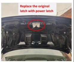
16. Replace the original latch with power latch and adjust it to the locked state.
