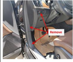
. Remove the indicated trim panels, door sill panel and 2. Remove the rear left side door sill panel and B-pillar trim panel.
