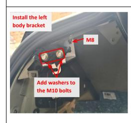
9. Install the left body bracket in the the way.
