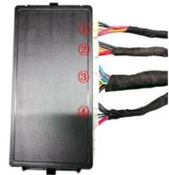
29. Insert the left and right strut wiring harnesses (1) (2),
