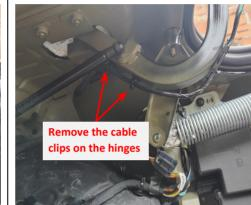
6.Remove the cable clips on the left and right hinges.
