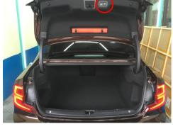
33. Fit the added tailgate switch in and reinstall all trim
