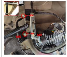
11. Insert the M6 bolt through the eye-bolt, insert the eye bolt through the bracket hole and secure them with | 12. Install the left tailgate bracket in the same way. M6 nut and M8 nut.
