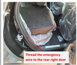
19. Thread the emergency wire to the rear right door and hide them under the door sill panel.
