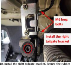
cylinder head screw at the bump stop position and thread the M6 bolts from the inner side to the other
