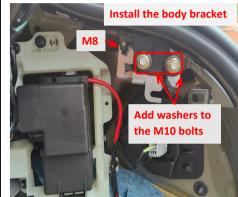
Install the right body bracket. Secure the M8 bolt first, then secure the M10 bolts with washers.
