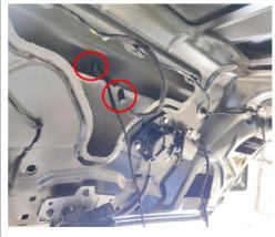
18. Connect the plugs of the lock signal harness to the plugs of original tailgate switch.
