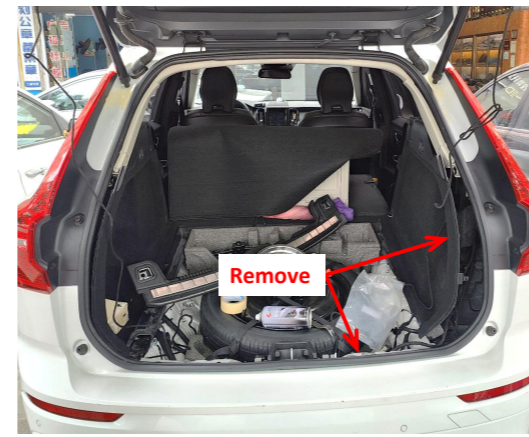
4. Remove the trunk floor mat, door sill panel and the trim panel on the left right of the trunk.
