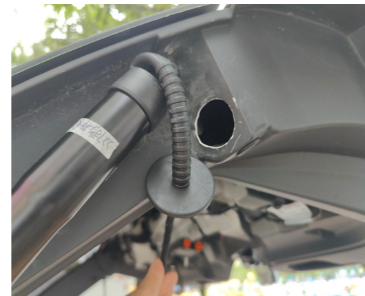
14. Plug the hole with the rubber plug on the strut; both sides are the same.
