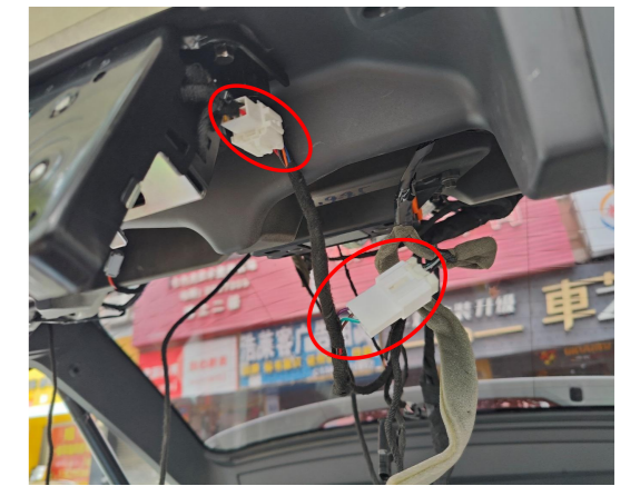
6. Connect the lock signal harness to the plugs of the power latch.
