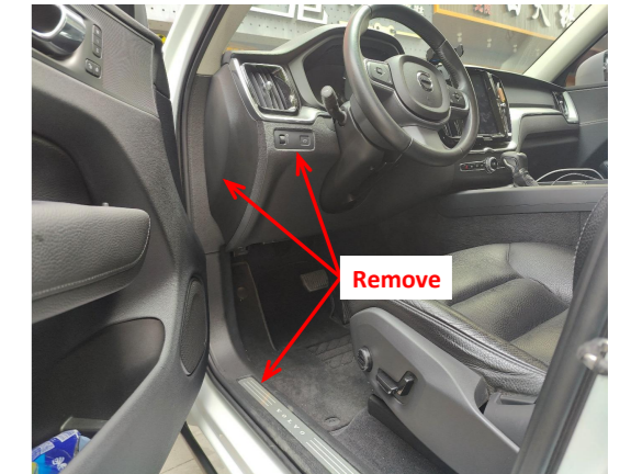
1. Remove the front left side door sill panel and switch panel.
