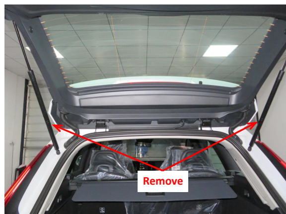
12. Remove the original gas struts.
