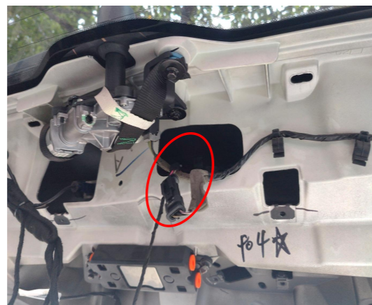
8. Route the lock signal harness to the right side of the trunk (no plug connection for now).
