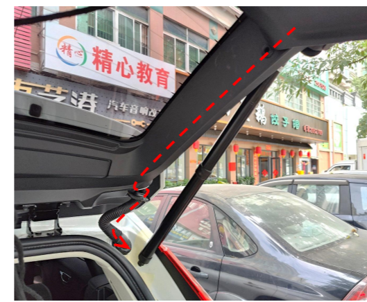
9. Thread the lock signal harness through the rubber tube on the right side.
