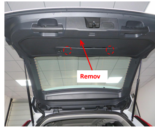
3. Remove the tailgate trim panel and pay attention to the fasteners.
