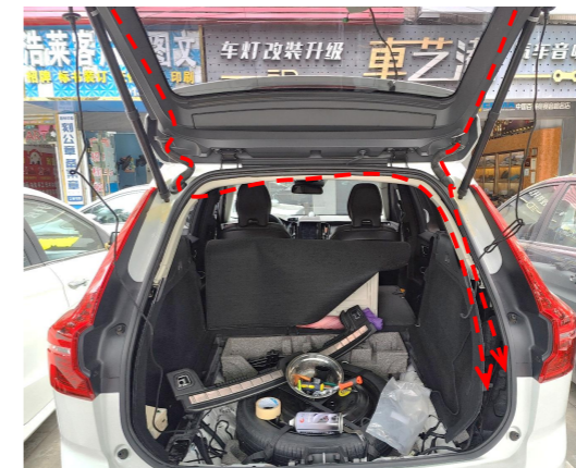
15. Route the left and right strut wiring harnesses to the right side of the trunk.
