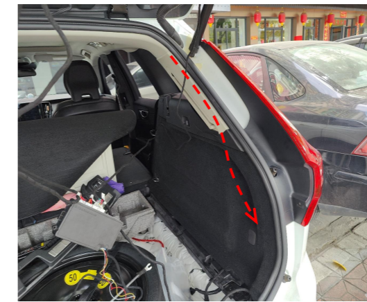
10. Route the lock signal harness to the bottom right of the trunk.
