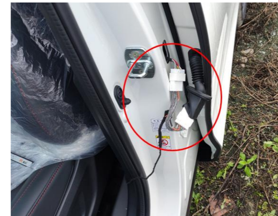
20. Connect to the B-pillar plugs at rear left B-pillar.
