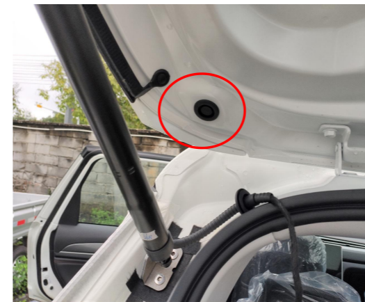
9. Thread the strut wiring harness through the indicated hole, the same on both sides.
