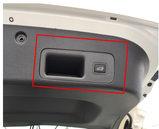
27. Install the added tailgate switch and reinstall all the trim panels (remove the original small cover).
