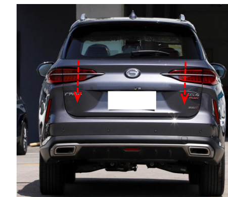
26. Press the added tailgate switch to close the tailgate once, the system completes initialization, and then test each function of the electric tailgate.
