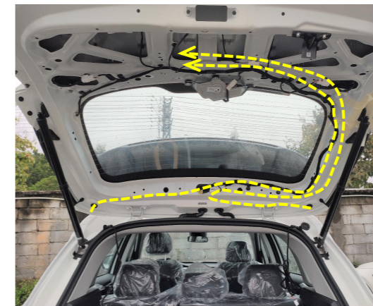
10. Route the strut wiring harnesses as indicated.
