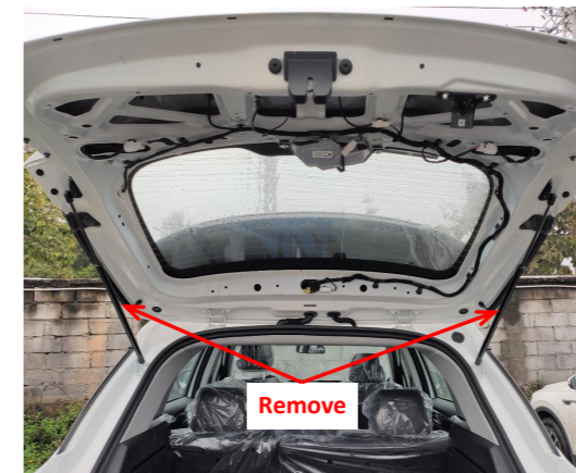
5. Remove the original gas struts.
