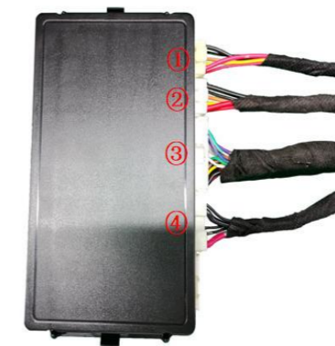
25. Insert the left and right strut wiring harnesses ①②, lock signal harness ③, and power harness ④ into the ECU in sequence.
