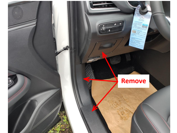
1. Remove the indicated driver side trim panels and storage box.
