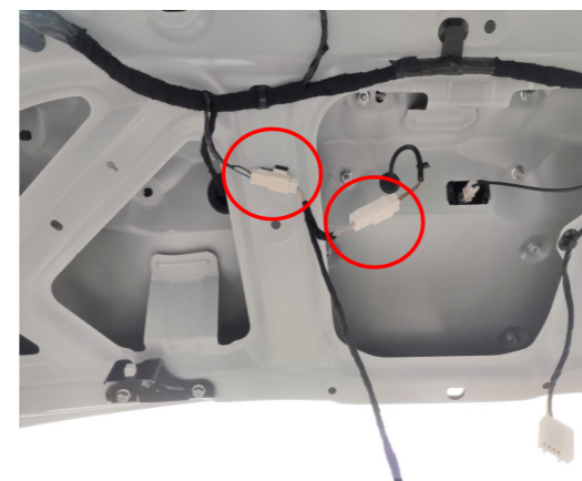
14. Connect the plugs of the lock signal harness to the plugs of original tailgate switch.
