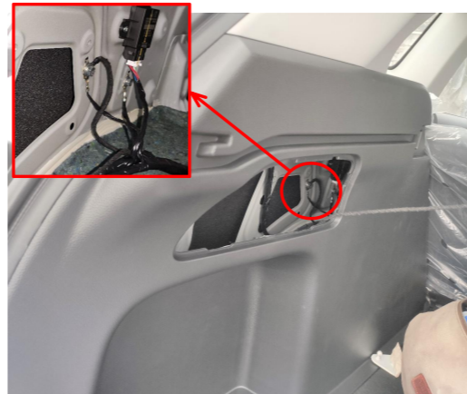
19. Ground at the indicated position on the left side of the trunk.
