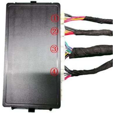
22. Insert the strut wiring harnesses ①②, lock signal harness ③, and power harness ④ into the ECU in sequence, and then fit the ECU into its bracket.
