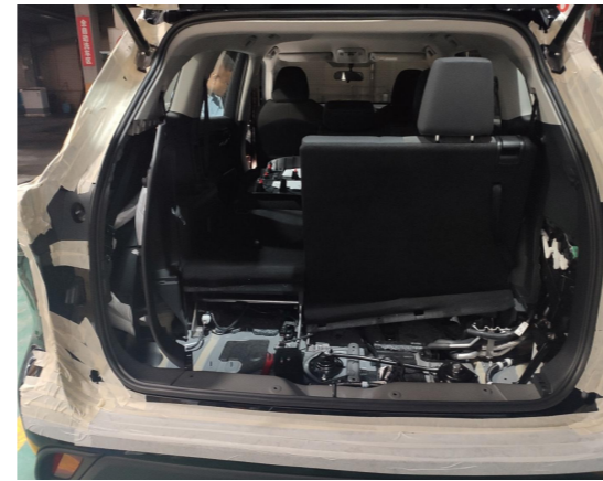
4. Remove the door sill panel, storage box and left side trim panel from the trunk.
