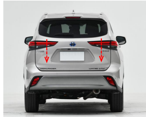
23. Press the added tailgate switch to open and close the tailgate once, the system completes initialization, and then test the functions of the electric tailgate.
