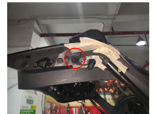
12. Thread the strut wiring harness through the indicated hole and plug the hole with the rubber plug. Both sides are the same.
