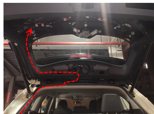
13. Route the power harness to the tailgate (do not connect plugs before inserting terminals into wiring harness connector).
