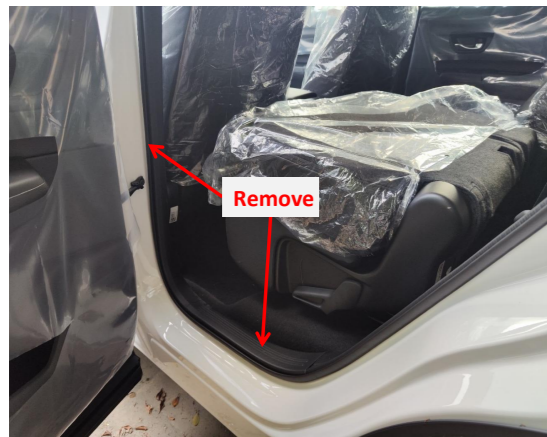
2. Remove the B-pillar trim panel and rear left door sill panel.
