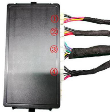
28. Insert the strut wiring harness ①, lock signal harness ③, and power harness ④ into the ECU in sequence and mount the ECU onto its bracket.
