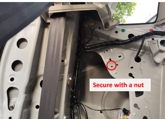
27. Secure the ECU at the left side of the trunk.
