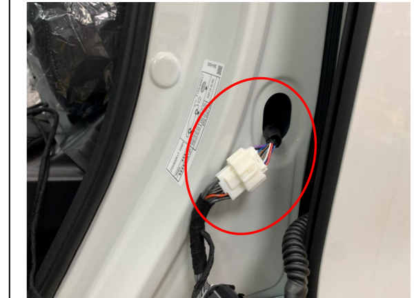
21. Connect the power harness to the indicated B-pillar signal plugs.
