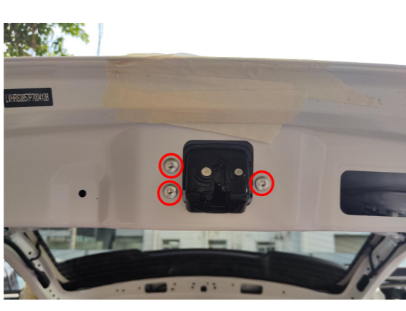
13. Remove the original latch and install the power latch.
