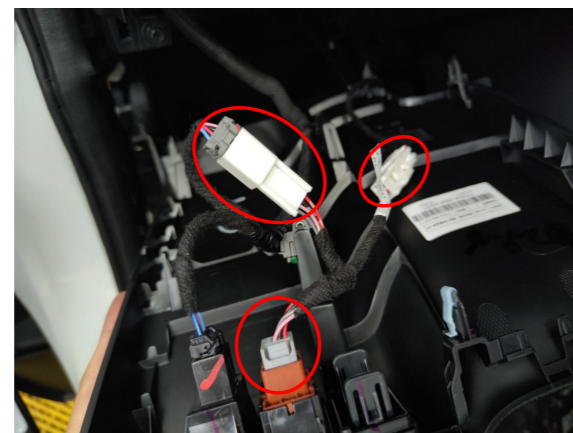
23. Connect the power harness to the plugs of the front switch behind the panel.
