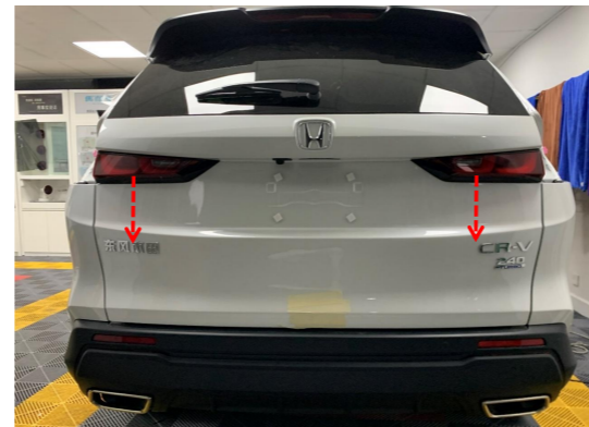
29. Press the added tailgate switch button once to initialize the system once and then test each function of the electric tailgate.
