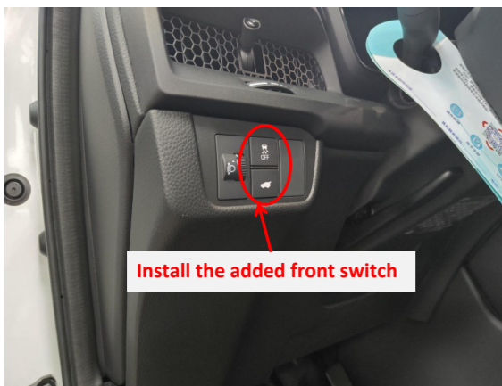
22. Remove the blank button and install the added front switch button.
