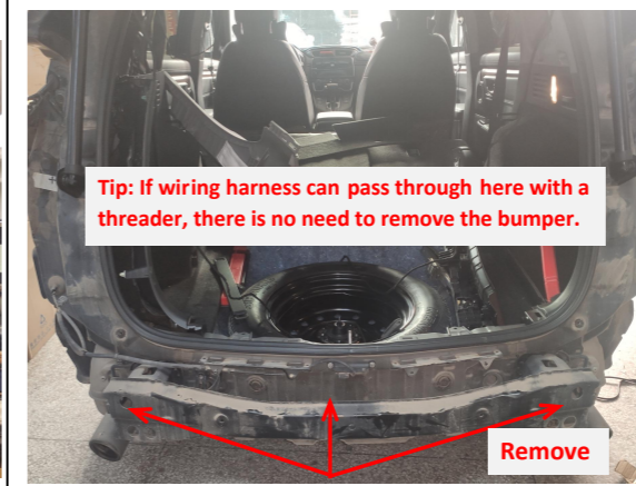
5. Remove the bumpers (if wiring harness can pass through here with a threader, there is no need to remove the bumper).
