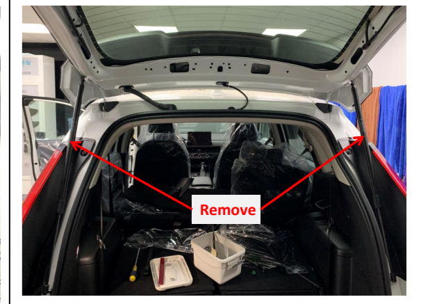
6. Remove the gas struts.
