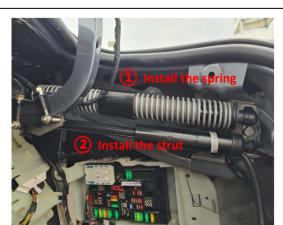
12. Install the right spring and strut in the same way.
