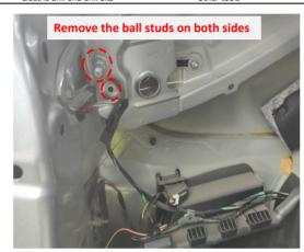
I. Remove the ball stud on both sides and install the bracket 5. Install the left body bracket. Insert the bolt with a handle on that hole and the hole under it.
