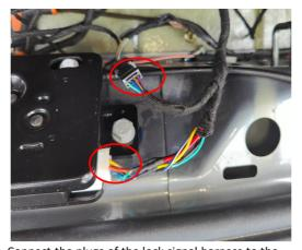
19. Connect the plugs of the lock signal harness to the power latch.
