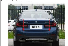
27. Press the tailgate switch buttons to close and open the tailgate once to complete the initialization, and then test each function of the electric tailgate.
