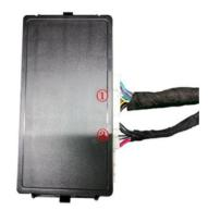
24. Insert the Lock signal harness ①, power harness ② into the ECU. Manually adjust the power latch to the locked state, press he original tailgate switch button and see whether the latch can be locked. If not, check whether the plugs are properly connected.
