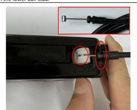
13. Unfasten the unlock arm of the power latch for installing 14. Put the cylindrical head of the cable into the reserve hole of the unlock arm and secure it at the indicated slot.
