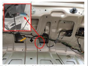
20. Connect the plug of the lock signal harness to the tailgate handle switch.
