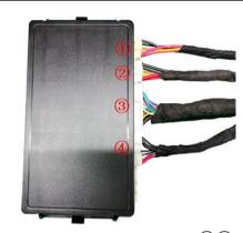
26. Insert the left and right strut wiring harnesses (1)(2), lock signal harness (3), and power harness (4) into the ECU in sequence.
