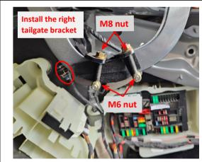
11. Install the right tailgate bracket on the right hinge in the
