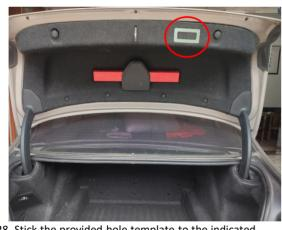
28. Stick the provided hole template to the indicated position and open a hole for the added tailgate switch.
