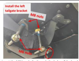
8. Insert the M6 long bolts through the holes of the bracket into the holes of eye bolts, then insert the eye bolts into the upper holes of the bracket and secure them with nuts.
