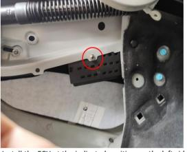
25. Install the ECU at the indicated position on the left side of the trunk.
