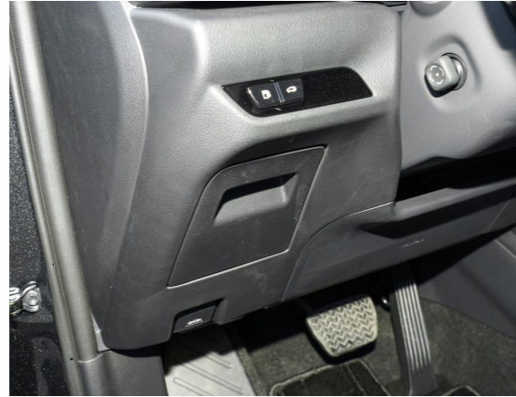
(Optional) Find an appropriate position in the driver's area, drill a \phi 21\text{mm} hole and install the added front switch.
