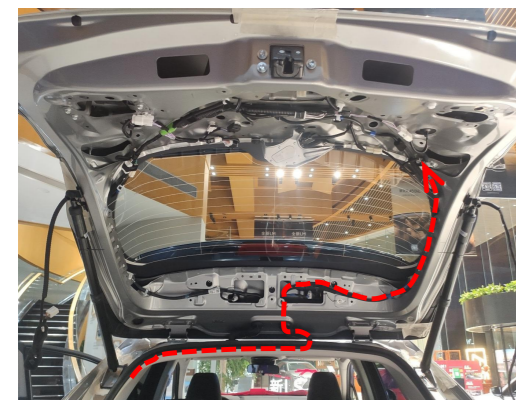
12. Thread the power harness to the tailgate (do not connect plugs before inserting terminals into wiring harness connector).
