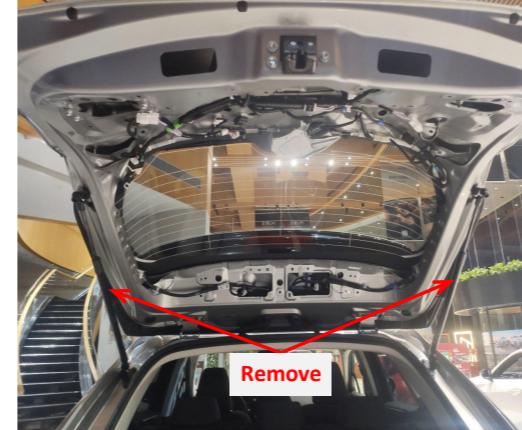
4. Remove the original gas struts.
