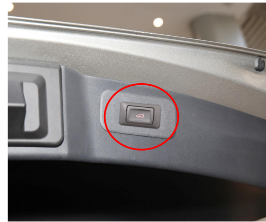
22. Install all the trim panels back and install the added tailgate switch.
