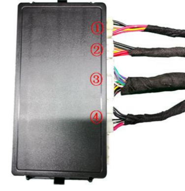
20. Insert the strut wiring harnesses ①②, lock signal harness ③, and power harness ④ into the ECU in sequence, and mount the ECU onto its bracket.
