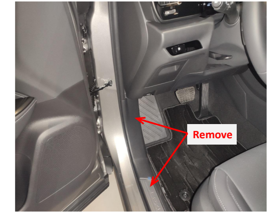
1. Remove the front left side trim panel and door sill panel.
