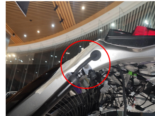
8. Remove the circled rubber plug from the tailgate to allow the strut wiring harness to pass through and then plug it back. Both sides are the same.
