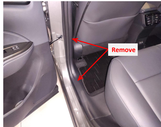
2. Remove the rear left side B-pillar trim panel and door sill panel.
