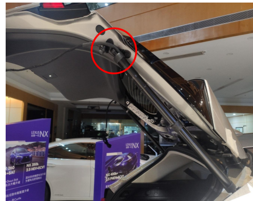
7. Install the electric struts, L on the left and R on the right (the first letter of the strut code), making sure the ends with wiring harnesses are on the tailgate.
