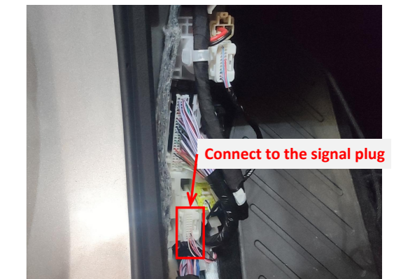
11. Connect the lock signal harness to the plugs of original tailgate switch and the added tailgate switch.
