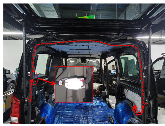
13. Route the strut wiring harnesses to the right side of the trunk as indicated.
