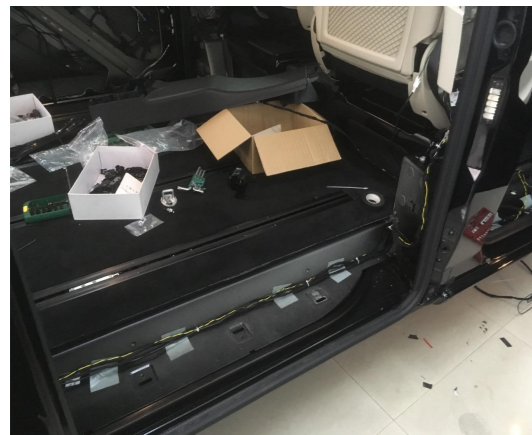
2. Remove the right front door sill panel and the right middle door sill panel.
