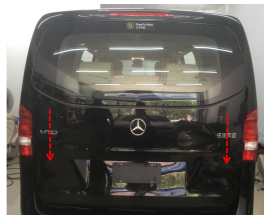
28. Press the added tailgate switch to close the tailgate once, and then test each function of the electric tailgate.
