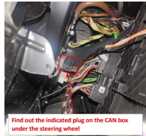
23. Find out the indicated CAN box under the steering wheel and plug in the signal plug.
