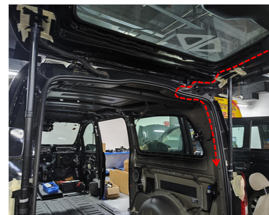
14. Route the lock signal harness to the right side of the trunk as indicated.
