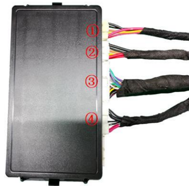
27. Insert the strut wiring harnesses ①②, lock signal harness ③, and power harness ④ into the ECU in sequence and then fit the ECU onto its bracket.
