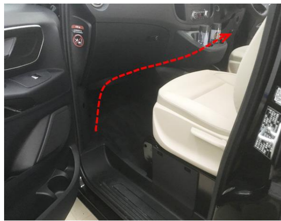
22. Thread CAN signal harness to the driver's area.
