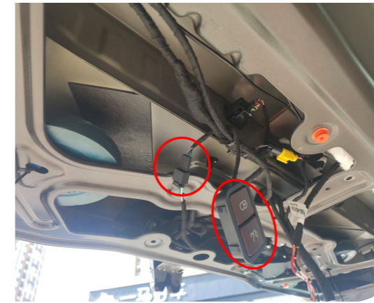
20. Connect the plug of the lock signal harness to the added tailgate switch.
