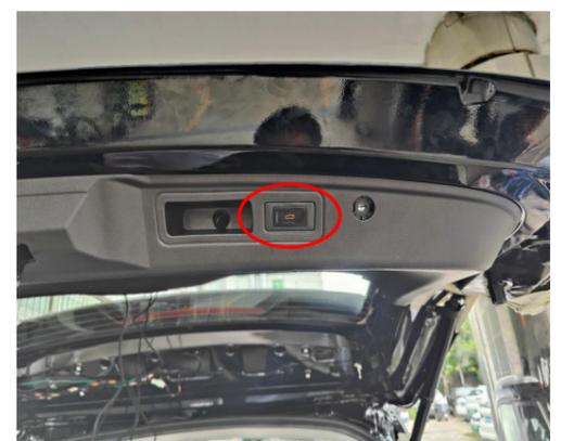
28. Reinstall all the trim panels and install the added tailgate switch(remove the original small cover).
