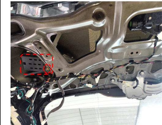
25. Secure the ECU bracket at the indicated position of the tailgate.
