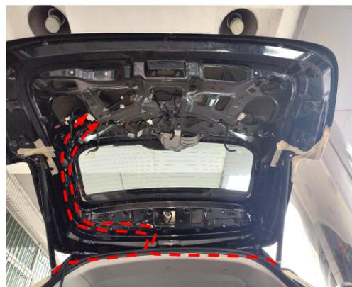
12. Route the left and right strut wiring harness to the tailgate.
