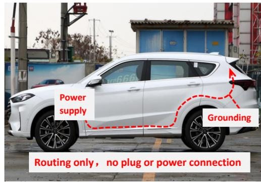
18. Route the power harness (if you need to install the added front switch, route the switch wiring harness in the same way).
