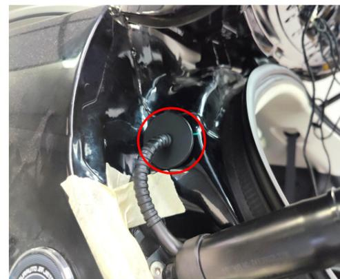
14. Plug the hole securely and leave a certain length of the rubber tube outside to prevent wire harness from being pulled.
