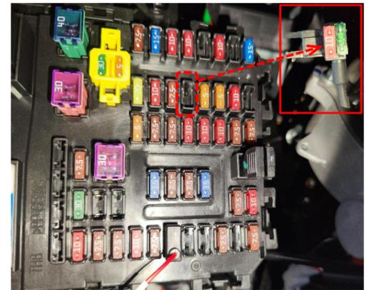
23. Move the indicated fuse from the fuse box to the fuse tap.
