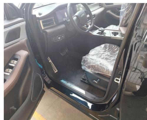
(Optional) Find an appropriate position in the driver's area, drill a  $\phi 21\text{mm}$  hole and install the added front switch.
