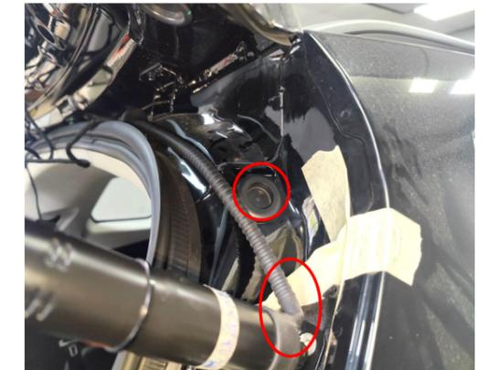
11. Thread the strut wiring harness through the indicated hole to the tailgate, the same on both sides.
