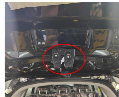
15. Remove the original latch and install the power latch with original screws.
