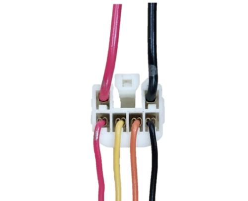
13. Insert the strut wiring harness terminals into the wiring harness connector as indicated above.
