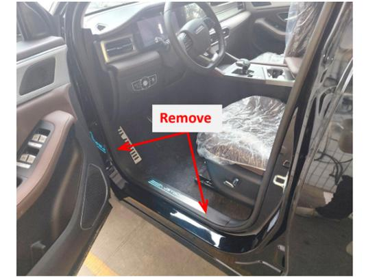
1. Remove the driver side trim panel and door sill panel.
