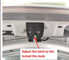
17. Install the power latch with original screws. Manually adjust the latch to the locked state to prevent accidental closing.
