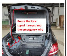
21. Route the lock signal harness and the emergency wire to the trunk along with the left hinge.
