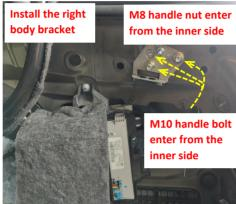
1. Install the left body bracket: thread the M8 handle nut 5. Install the right body bracket: thread the M8 handle nut to secure the bracket first and then thread the M10
