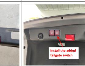
38. Reinstall all trim panels and install the added tailgate switch.
