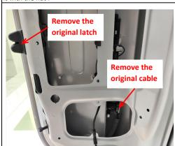
15. Remove the original latch and cable.
