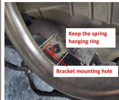
. On the right hinge, keep the spring hanging ring and only use the hole beside for securing the bracket.
