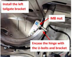
7. Encase the hinge with the U-bolt and bracket and tighten the bolt with the M8 nut.
