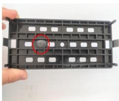
28. Remove the ECU, place a bolt on the bracket and mount the ECU onto its bracket.
