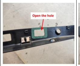
37. Fit the added switch in and check whether it can bounce back normally.
