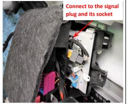
25. Connect to the signal plug behind the fuse box on the right side of the trunk.
