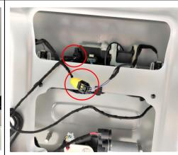
20. Connect the plugs of the lock signal harness to the plugs of original tailgate switch and the added tailgate switch.
