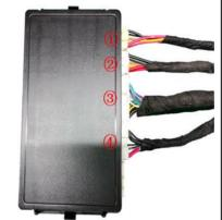
30. Insert the left and right strut wiring harnesses (1)(2), lock signal harness 3, and power harness 4 into the ECU in sequence.
