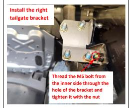
9. Install the right tailgate bracket: thread the M5 bolt through the bracket hole from the inner side and tighten t with the nut
