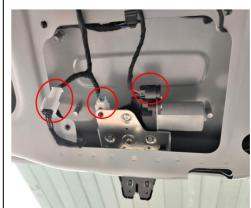
18. Install the emergency cable. (use the mechanical key 19. Connect the plugs of the lock signal harness to the plugs of the power latch.
