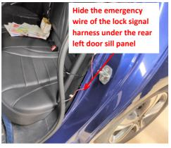
22. Thread the emergency wires of the lock signal harness to the rear left door and hide them under the trim panel.
