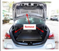
L. Remove the trim panels from the tailgate and trunk. 2. Remove the springs on both sides.
