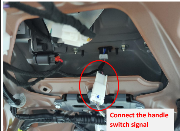
12. Connect the T-harness connectors of the lock signal harness to the tailgate handle switch.
