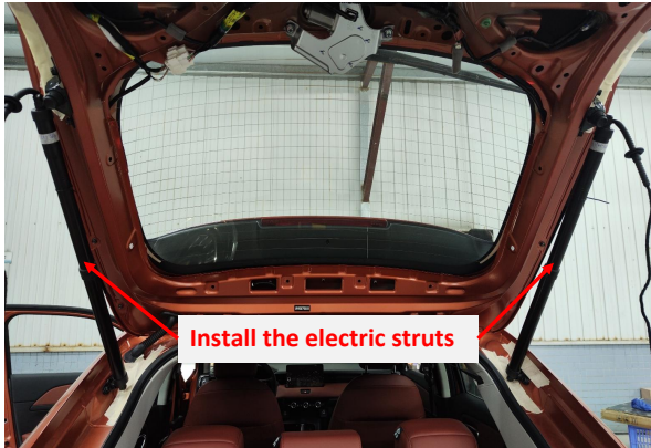
6. Install our electric struts.
