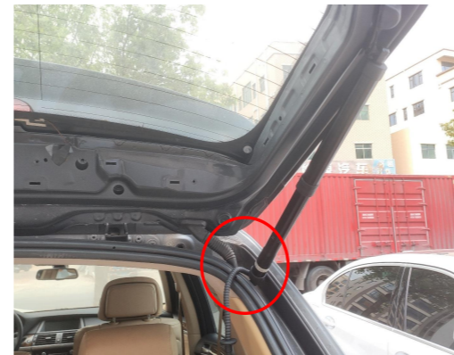
4. Install the electric struts, L on the left and R on the right (the first letter of the strut code), making sure the ends with wiring harnesses are on the car body.
