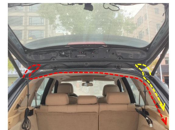
6. Route the strut wiring harnesses to the right side of the trunk.
