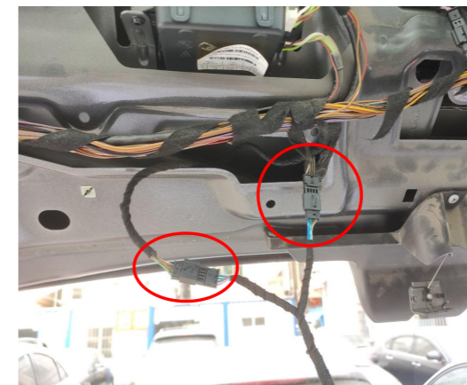
10. Connect the plugs of the lock signal harness to the plugs of the power latch.
