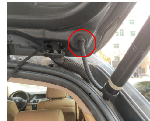
5. Thread the strut wiring harness through the indicated hole into tailgate and plug the hole with hole plug. Both sides are the same.
