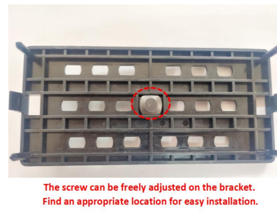
15. Place a screw on the ECU bracket and then mount the ECU onto its bracket.
