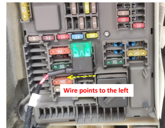
14. Plug the fuse tap into the fuse box with wire pointing to the left.
