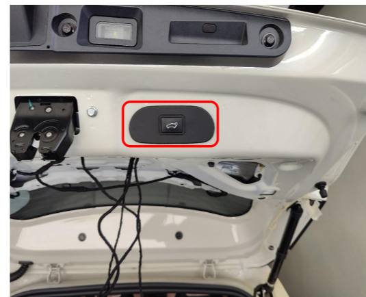
29. Install the added tailgate switch and reinstall all the trim panels.
