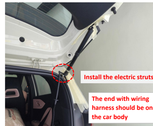
9. Install the electric struts, L on the left and R on the right (the first letter of the strut code).
