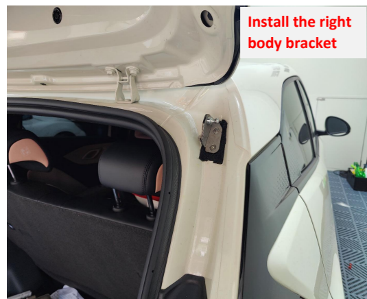
7. Replace the original bracket with our right body bracket.
