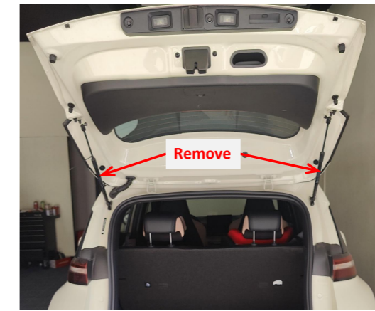
5. Remove the original gas struts.
