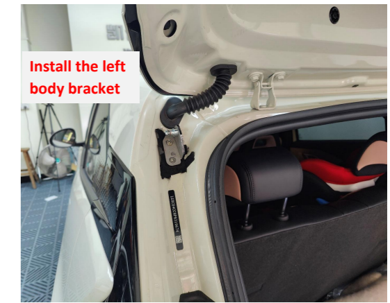
6. Replace the original bracket with our left body bracket.
