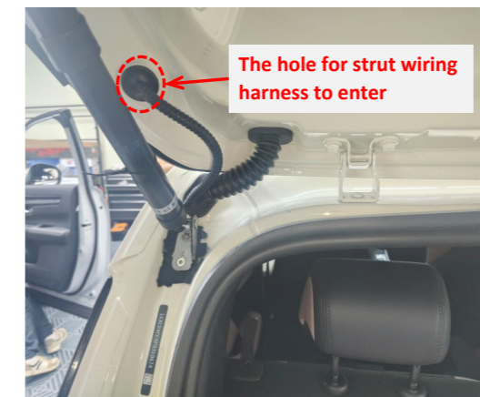
10. Remove the rubber plug from the indicated position to allow the strut wiring harness to pass through.
