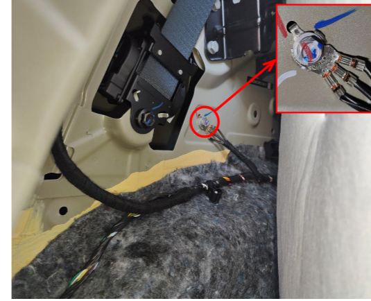
20. Ground at the indicated position on the left side of the trunk.
