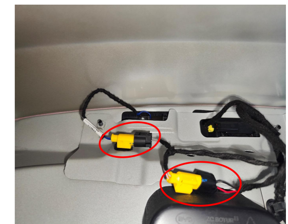
16. Connect the plugs of the lock signal harness to the plugs of original tailgate switch.
