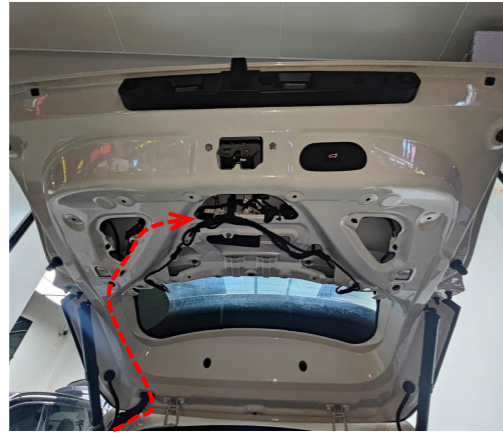
18. Thread the power harness to the tailgate.
