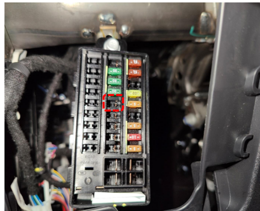
23. The fuse box is located under the storage box at the driver's area and the slot for power supply is indicated.
