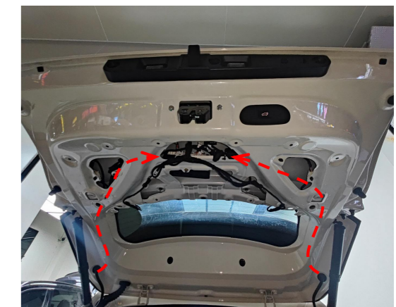
11. Route the left and right strut wiring harness as indicated.
