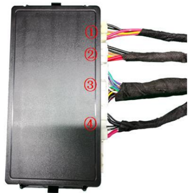
27. Insert the left and right strut wiring harnesses ① ②, lock signal harness ③, and power harness ④ into the ECU in sequence.
