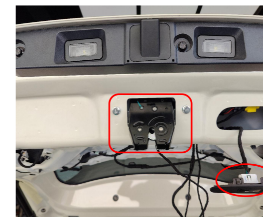
15. Install the power latch and connect the plug of the lock signal harness to the added tailgate switch.
