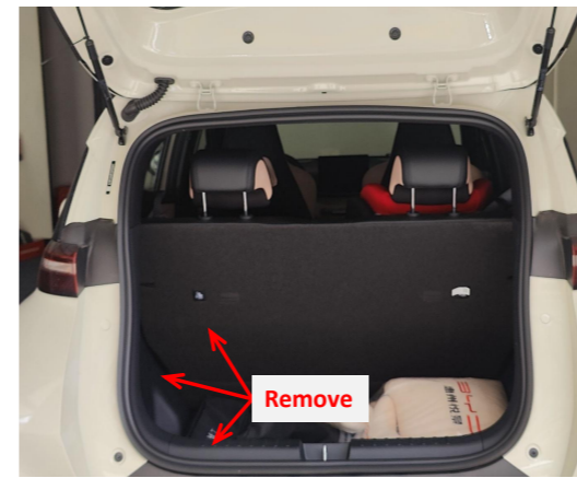
4. Take out the trunk floor mat and remove the indicated trim panels.
