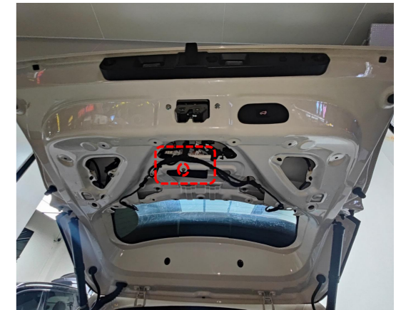
26. Secure the ECU at the indicated position with a nut and make sure the sockets side face outward.
