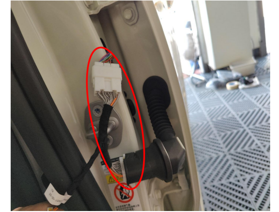
21. Connect to the signal plugs at the rear left B-pillar.
