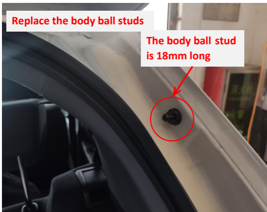
7. Replace the left and right body ball studs.
