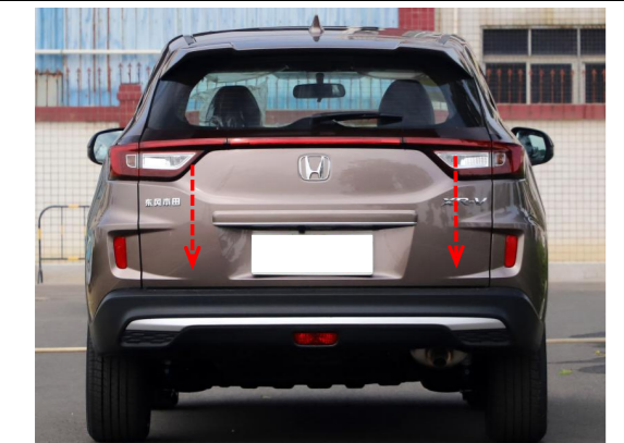
27. Press the added tailgate switch button to close the tailgate once for initializing the system and then test each function of the electric tailgate.
