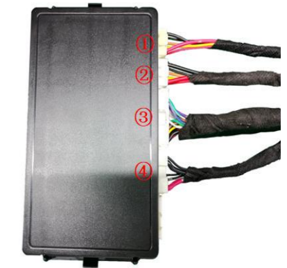
26. Insert the strut wiring harnesses ①②, lock signal harness ③, and power harness ④ into the ECU in sequence and mount the ECU onto its bracket.
