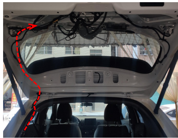
17. Route the power harness to the tailgate.
