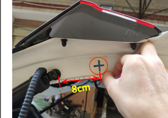
10. Drill a hole at the indicated position with a \phi 21\text{mm} drill bit to allow the strut wiring harness to pass through. Both sides are the same.
