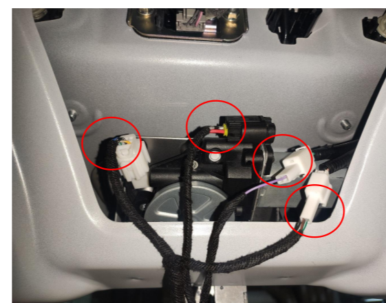
14. Connect the plugs of the lock signal harness to the plugs of the power latch.
