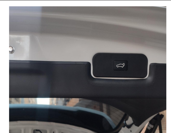
28. Reinstall all trim panels and and install the added tailgate switch.
