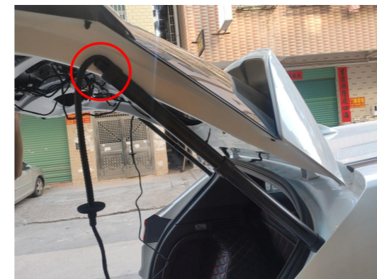
9. Install the electric struts, L on the left R on the right (the first letter of the strut code), making sure the the ends with wiring harnesses are on the tailgate.
