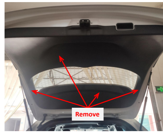
3. Remove the tailgate trim panels.
