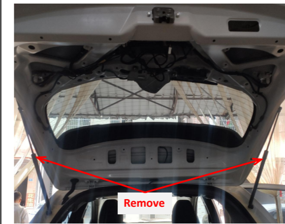
5. Remove the original gas struts.
