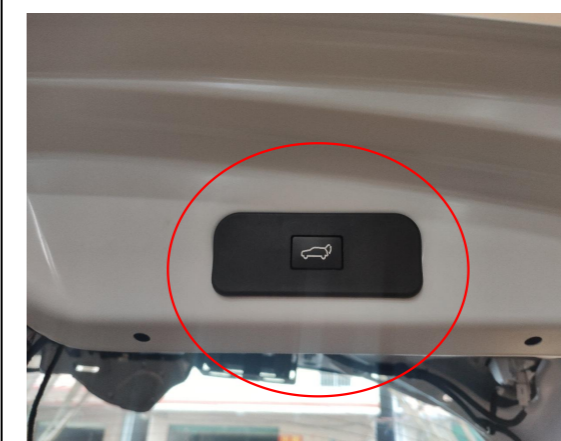
15. Remove the original tailgate handle and install the added tailgate switch.
