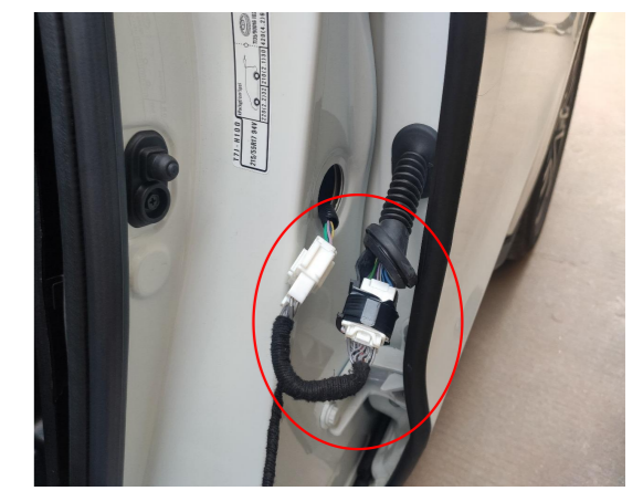
21. Connect the plugs of the power harness to the indicated plugs on the rear left side B-pillar.
