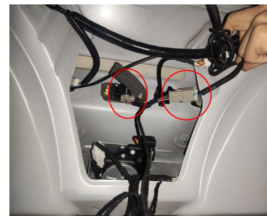
13. Connect the plugs of the lock signal harness to the plugs of the original tailgate switch.
