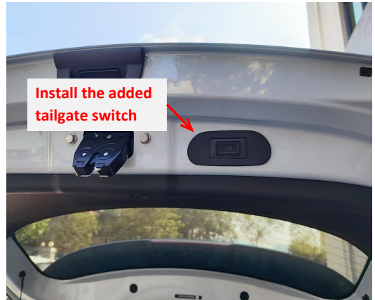
31. Reinstall all trim panels and install the added tailgate switch.
