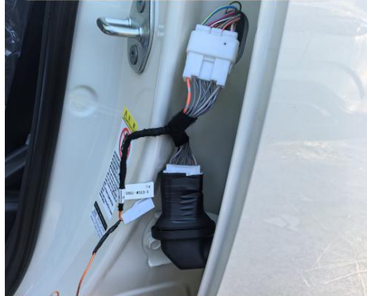
24-1. If there is no OBD plug at the driver's area, connect to the B-pillar signal plugs.
