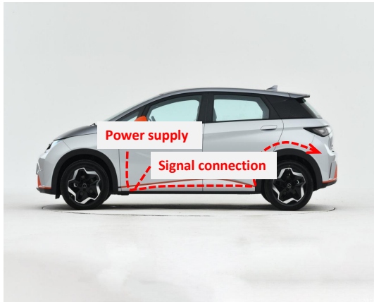
20. Route the power harness (wiring only, no plug or power connection).
