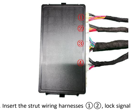
29. Insert the strut wiring harnesses ①②, lock signal harness ③, and power harness ④ into the ECU in sequence.
