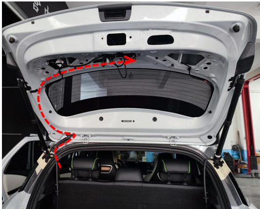
21. Route the power harness to the tailgate.
