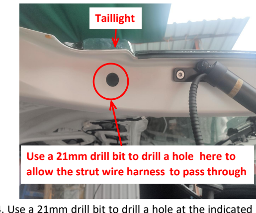
9. Drill a hole at the left side of the tailgate and for the left tailgate bracket.
