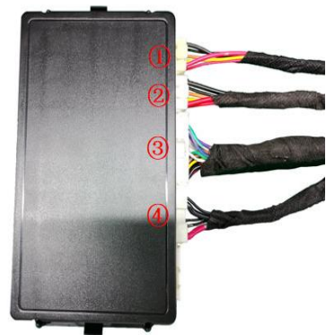
32. Insert the strut wiring harnesses ①②, lock signal harness ③, and power harness ④ into the ECU in sequence, and mount the ECU on its bracket.
