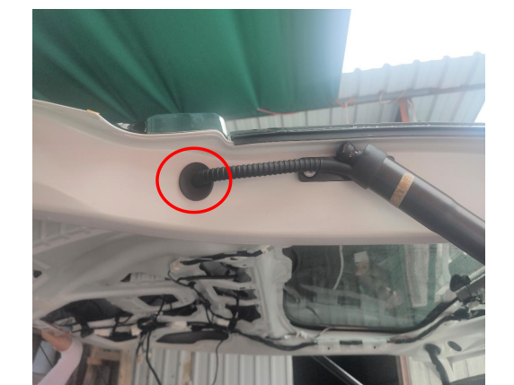
16. Plug the holes on the left and right sides of the tailgate with the hole plugs.
