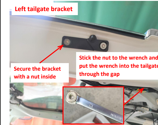
10. Install the bracket at the left side of the tailgate and fasten the other end of the bracket with a nut.
