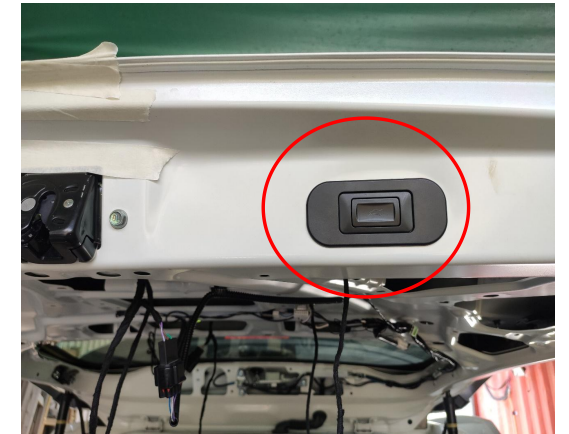
21. Remove the original small panel from the tailgate and install the added tailgate switch.
