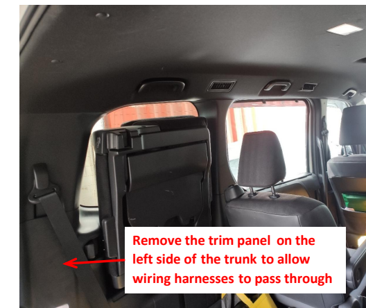
5. Remove the trim panel on the left side of the trunk to allow wiring harnesses to pass through.
