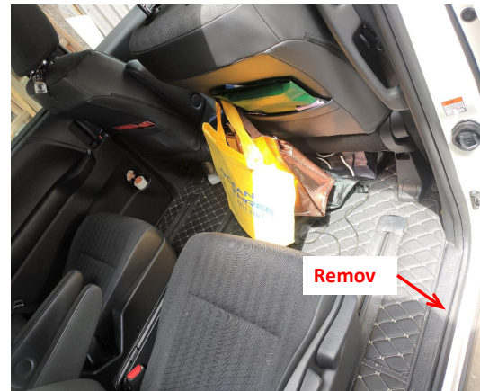
3. Remove the rear right side door sill panel.
