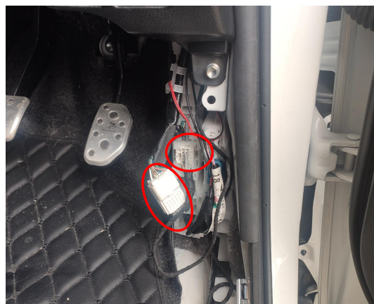
29. Connect the signal plugs of the power harness to the indicated plug and its socket beside the pedals.
