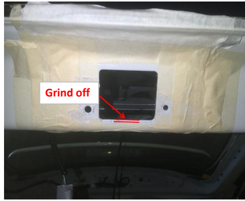
17. Remove the original latch and try to install our power latch. If there is any interference, grind off the lower edge of the hole.
