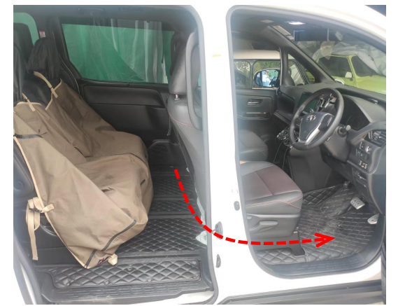
26. Route the plugs of the front switch wiring harness and the signal plugs to the driver's position.
