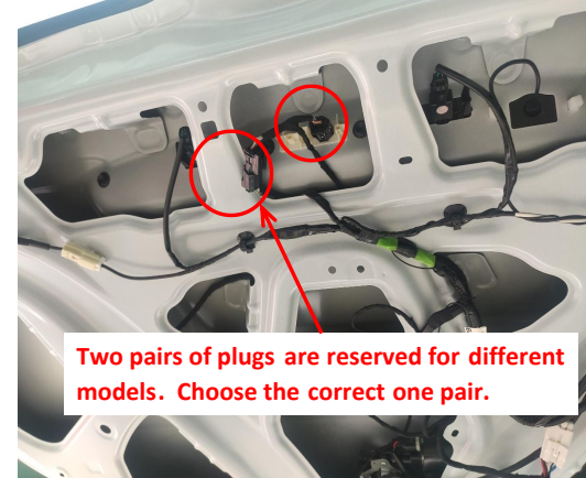
20. Connect the plugs of the lock signal harness to the plugs of the original tailgate switch.
