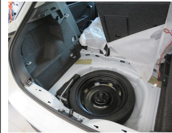
5. Take out the trunk floor mat and the trim panel on the left side.
