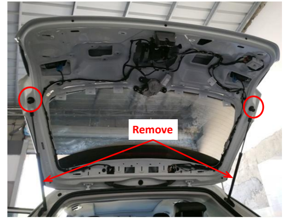
6. Remove the gas struts and the bump stops.
