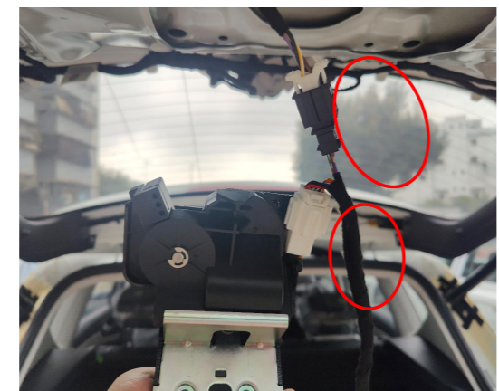
13. Connect the plugs of the lock signal harness to the power latch.
