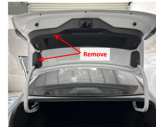
5. Remove the tailgate trim panels.
