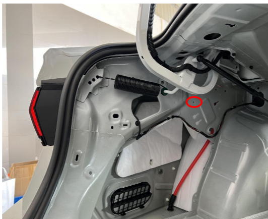
28. Secure the ECU at the indicated position with a nut.
