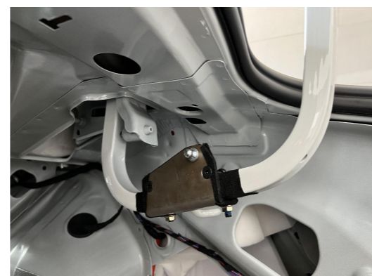
14. Tighten the nuts on those bolts.
