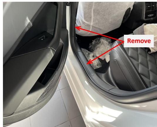
2. Remove the rear left door sill panel and B-pillar trim panel.
