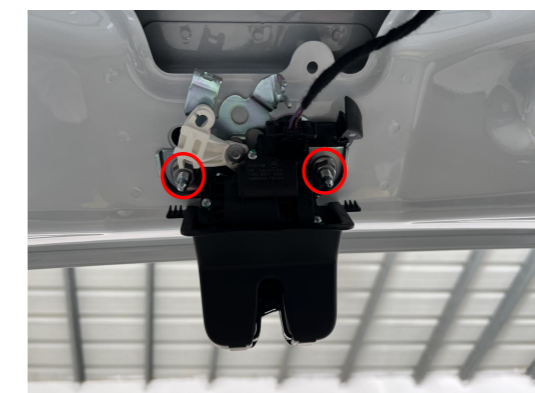
15. Remove the original latch.
