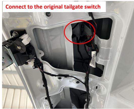
18. Connect the plugs of the lock signal harness to the plugs of the original tailgate switch.
