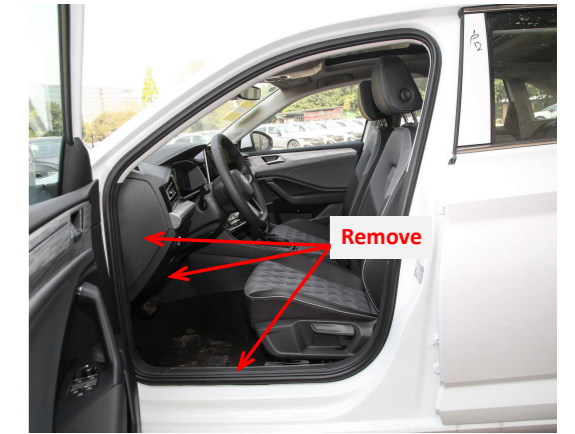
1. Remove the front left side door sill panel and the trim panels of the fuse box.
