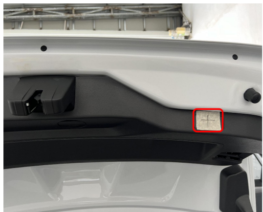
32. Stick the hole template to the indicated position and open a hole for the added tailgate switch.
