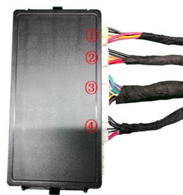
29. Insert the left and right strut wiring harnesses ①②, lock signal harness ③, and power harness ④ into the ECU in sequence.
