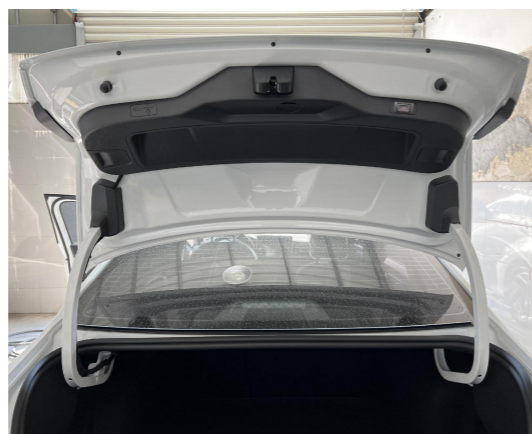
33. Install the added tailgate switch and reinstall all trim panels.
