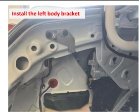
6. Install the left body bracket. Secure the bracket with the M10 hex socket bolt and two nuts with handle.
