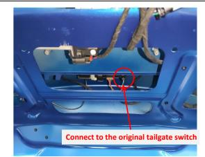
15. Connect the plugs of the lock signal harness to the plugs | 16. Connect the plugs of the lock signal harness to the plugs of original tailgate switch.
