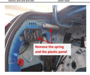
4. Remove the spring and the plastic panel.
