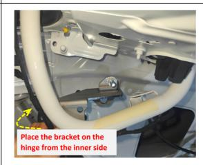
9. Place the bracket on the hinge from the inner side.
