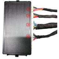
25. Insert the left and right strut wiring harnesses (1)(2), lock signal harness (3), and power harness (4) into the ECU lin seguence.
