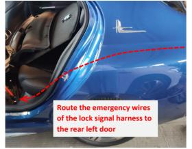
18. Route the emergency wires of the lock signal harness to 19. Route the power harness (Routing only, no plug or the rear left door and hide them under the door sill panel.
