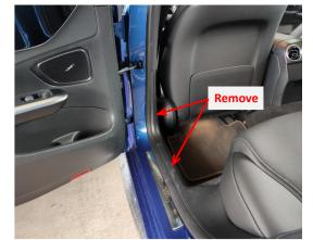
1. Remove the rear left door sill panel and B-pillar trim panel.
