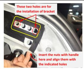
5. Locate the hole for the bracket, Insert the nuts with handle from the inner side and align them with the indicated holes
