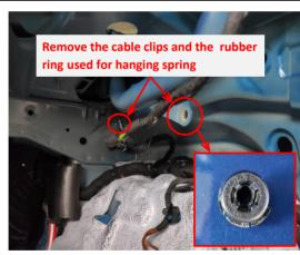
8. Remove the cable clips and the rubber ring used for hanging spring from the left and right hinges.
