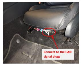
21. Connect to the CAN signal plugs under the driver's seat.
