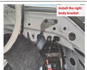
7. Install the right body bracket. Secure the bracket with the M10 hex socket bolt and two nuts with handle.
