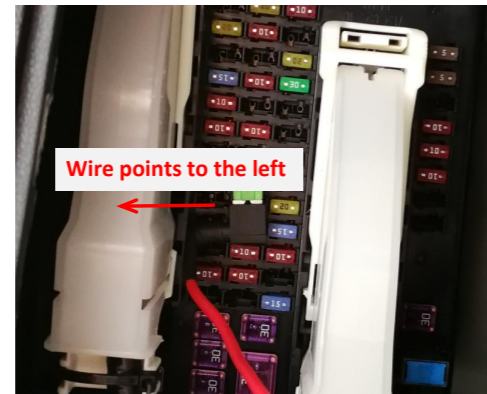
23. Move the original fuse from the slot to fuse tap, and then plug the fuse tap into the fuse box; pay attention to the direction.
