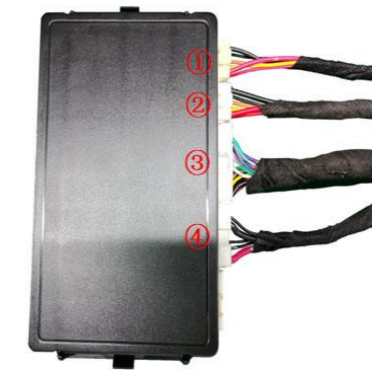
25. Insert the strut wiring harnesses ①②, lock signal harness ③, and power harness ④ into the ECU in sequence and then mount the ECU onto its bracket.
