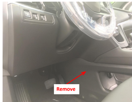
2. Remove the trim panel on the right side of the driver's seat.
