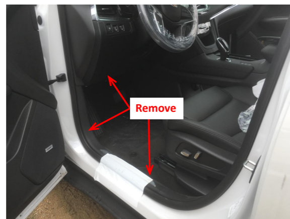
3. Remove the front left side trim panel, door sill panel and storage box.
