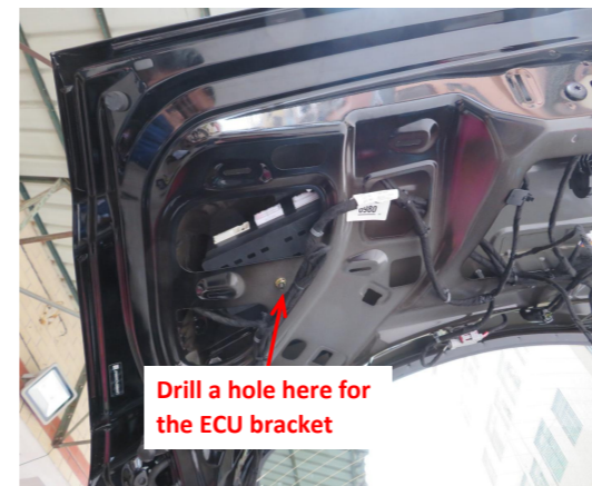
24. Drill a hole at the indicated position with a φ6mm drill bit for securing the ECU bracket.
