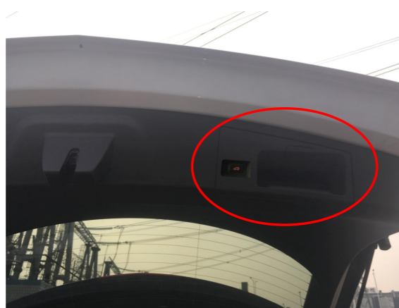
28. Reinstall all trim panels and replace the original tailgate handle with the added tailgate switch.
