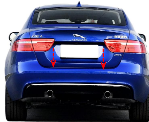
24. Close the tailgate to the position where the latch touches the striker, open and close the tailgate once, and test each function of the electric tailgate.
