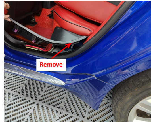
3. Remove the rear left door sill panel.
