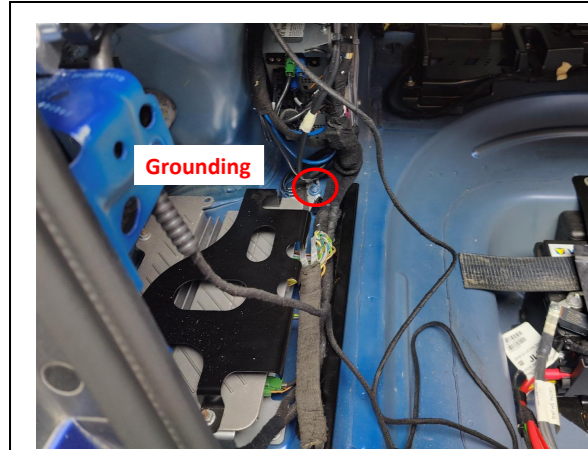
17. Ground at the indicated position on the left side of the trunk.
