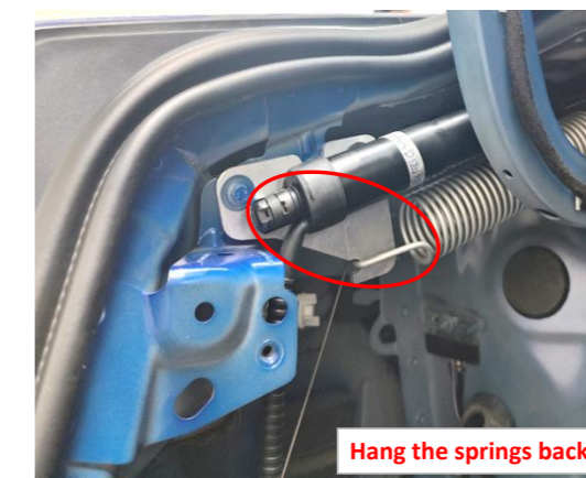
15. Install the left and right electric struts, L on the left, R on the right (the first letter of the strut code).
