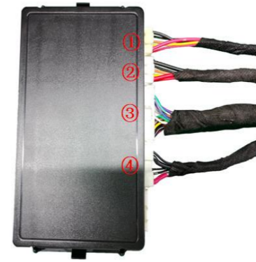
20. Insert the left and right strut wire harnesses ① ②, lock signal harness ③, and power harness ④ into the ECU in sequence.
