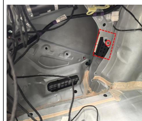
37. Secure the ECU at the indicated position.
