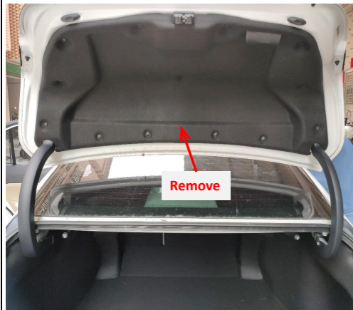
3. Remove the tailgate trim panel.
