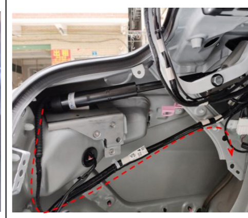
19. Route the left strut wiring harness along with original wires.
