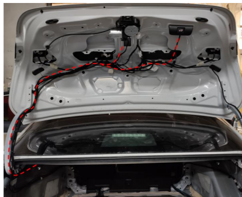
28. Route the lock signal harness to the tailgate along with original wires as indicated.
