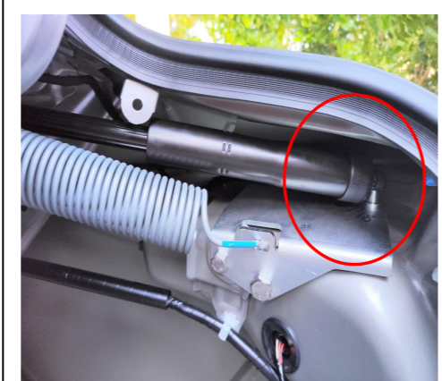
17. Install the electric struts, L on the left and R on the right (the first letter of the strut code), making sure the ends with wiring harnesses are on the car body.
