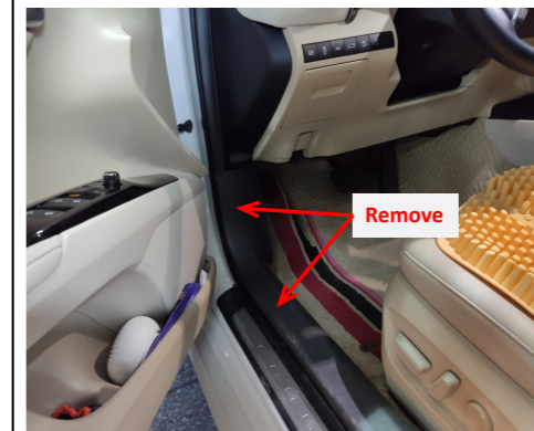
1. Remove the front left door sill panels.
