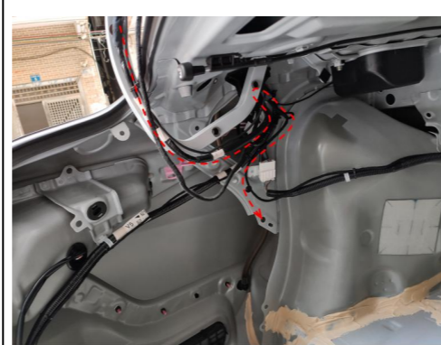
23. Install the power latch and manually adjust the latch to the locked state.
