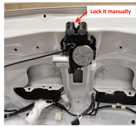
23. Install the power latch and manually adjust the latch to the locked state.
