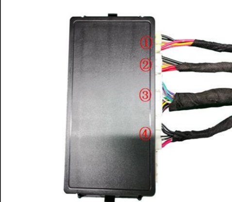
36. Insert the strut wiring harnesses ①②, lock signal harness ③, and power harness ④ into the ECU in sequence, mount the ECU onto its bracket.
