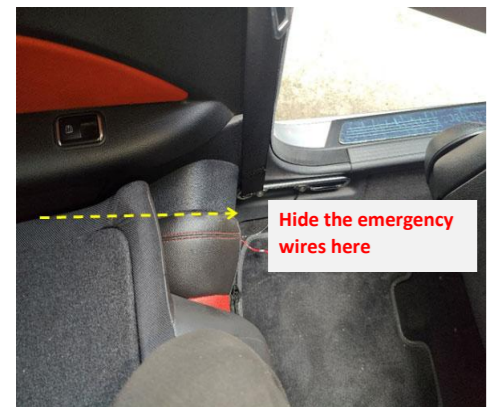
27. Route the two emergency wires of the latch as indicated above, wrap them together with the electric tape and then hide them under the rear left trim panel.
