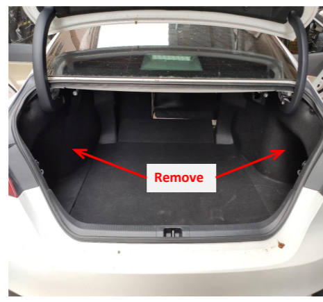
4. Take out the trunk floor mat and remove the trim panels on both sides of the trunk.
