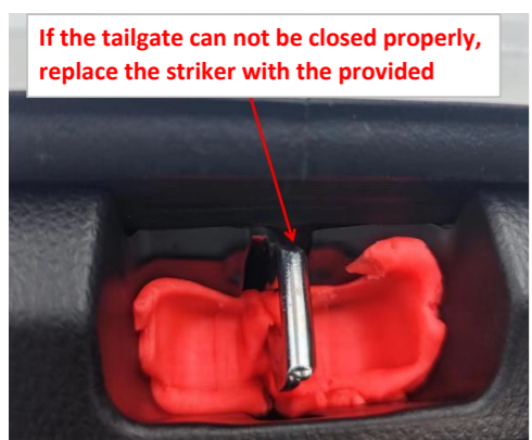
39. Check if the tailgate can be closed properly. If not, replace the striker with the provided one.
