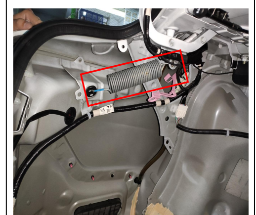
8. Remove the left and right springs from the trunk.
